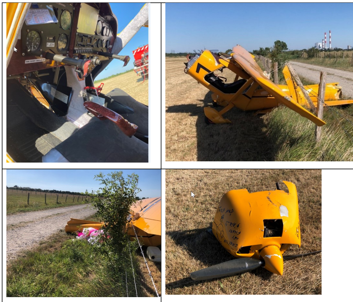
Figure 1: wreckage of microlight: ruptured wheels, airframe with parachute, separated engine mount
