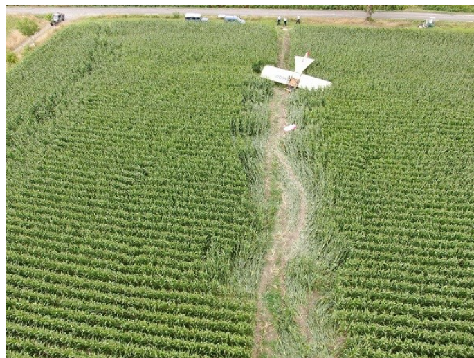
Figure 8: microlight dragged through the field by the parachute
