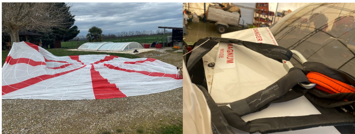
Figure 5: ballistic airframe parachute (on left-hand side: parachute canopy, on right-hand side: interfaces, harnesses)
