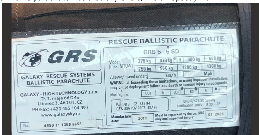
Figure 2: photograph of characteristics of ballistic airframe parachute (source: pilot)
