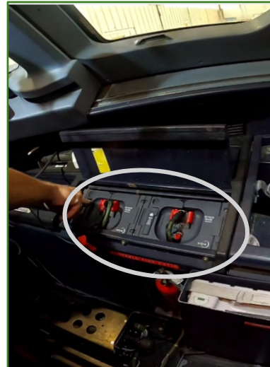
Oxygen mask storage boxes on commercial air transport aeroplane
