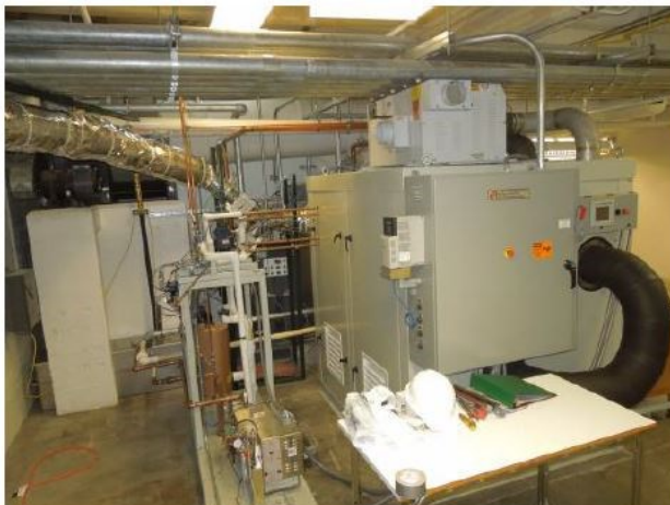
Figure 49: climatic condition reproducer used during the tests
