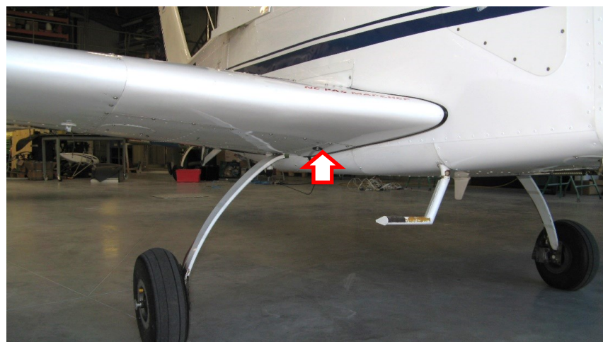
Figure 197: temperature and relative humidity measurement sensor Source: BEA
