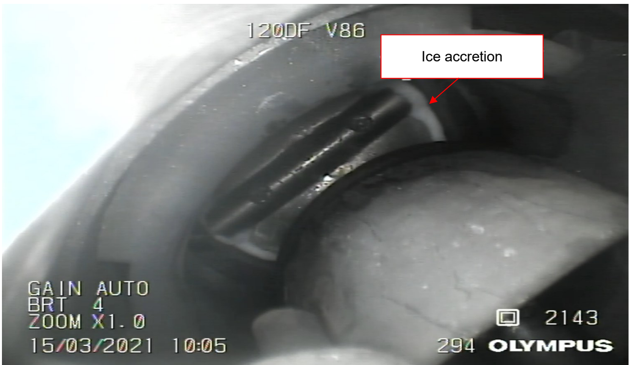
Figure 106: progress of icing => time designated t_0 + 5 \text{ min } 43 \text{ s} . Source: BEA
