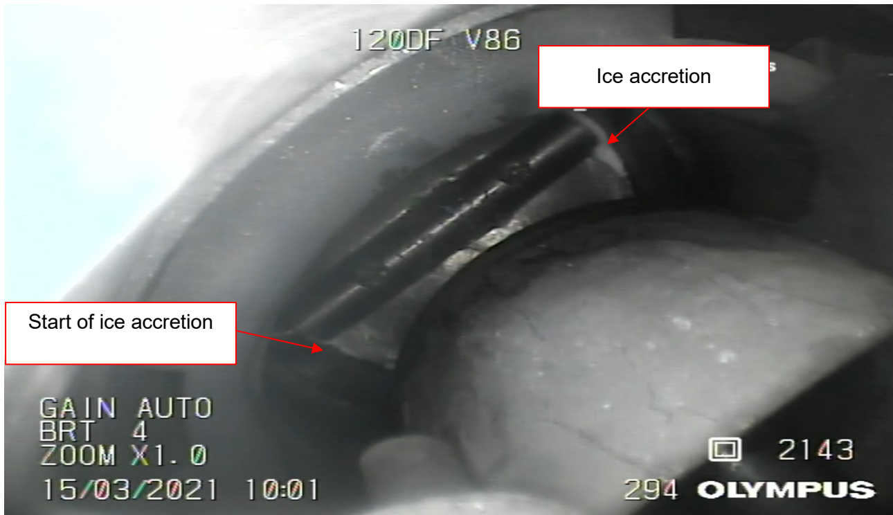
Figure 104: progress of icing => time designated t_0 + 2 \text{ min} Source: BEA
