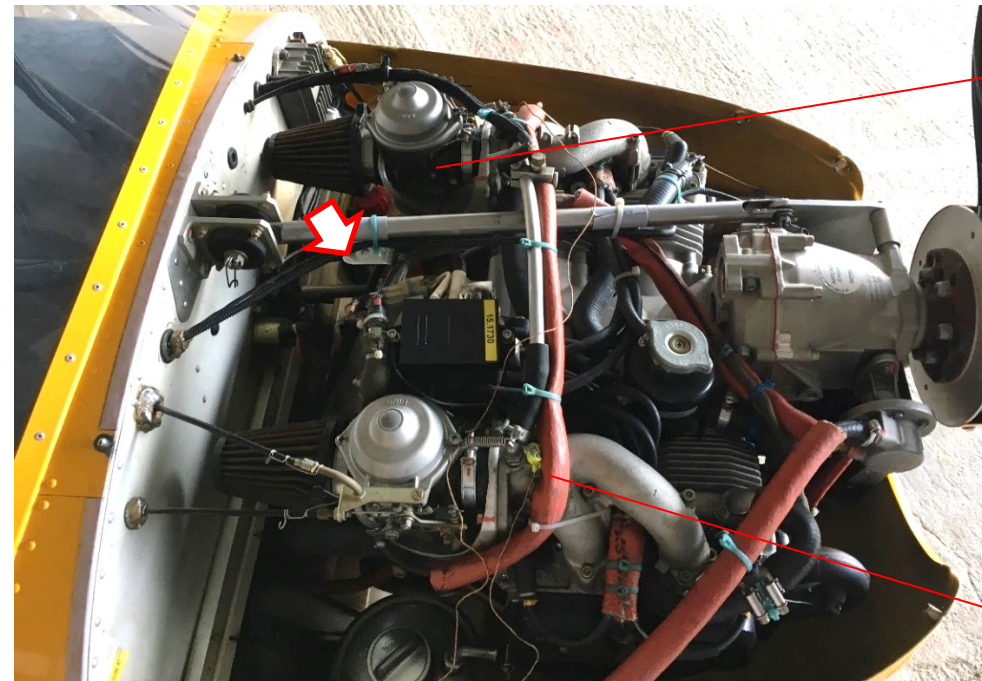
Figure 187: temperature/relative humidity sensor Source: BEA
