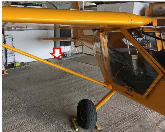
Figure 186: temperature/relative humidity sensor Source: BEA
