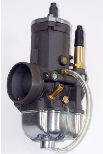
Figure 148: outside view of a Bing 54 carburettor Source: https://www.finesse-max.com/rotax/1015-pointeau-de-carburateur-bing-54.html
