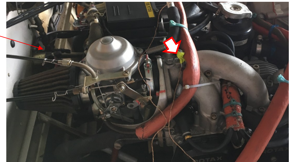
Figure 189: temperature sensor Source: BEA
