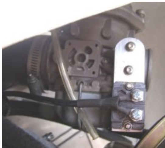
Figure 145: positioning of the heat resistor on the outer surface of the carburettor
