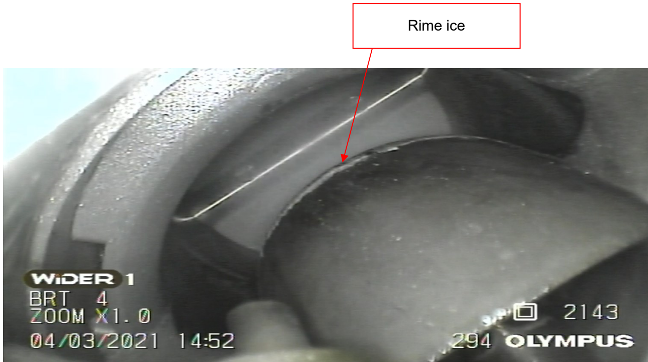
Figure 122: presence of rime ice on the outer surface of the venturi Source: BEA
