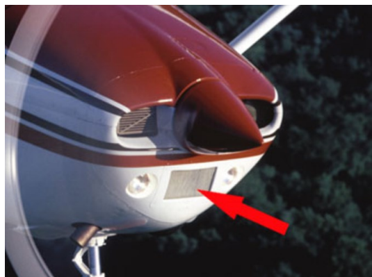
Figure 3: zone conducive to impact icing Source: aopa.com
