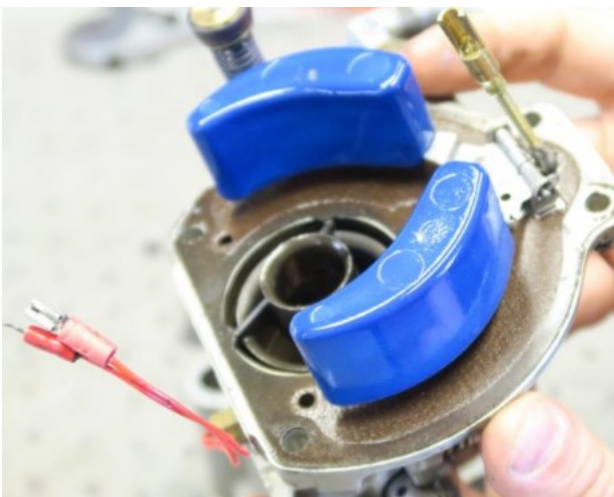
Figure 11: illustration of two floats interconnected by a metallic part Source: BEA
