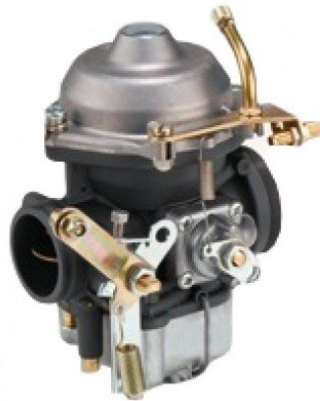
Figure 141: outside view of a Bing 64/3 carburettor
