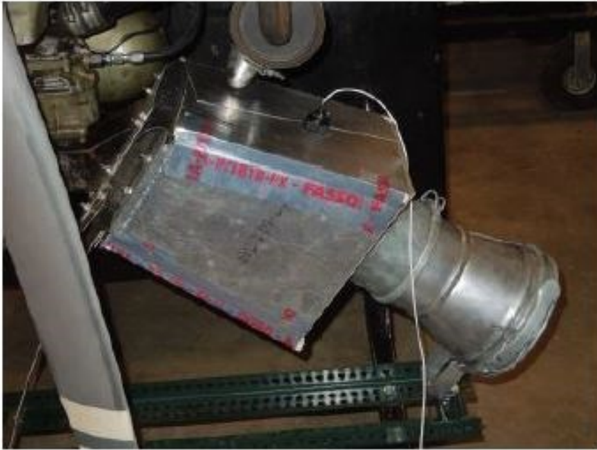
Figure 48: enclosure surrounding the carburettor to provide the required temperature and humidity conditions
