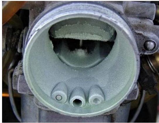
Figure 5: icing of a constant depression carburettor
