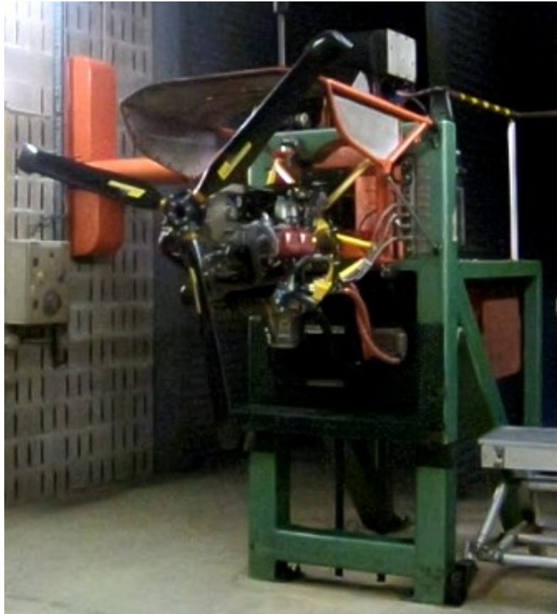
Figure 150: BEA Rotax 914 engine installed on the ENAC's Castenaudary test stand
