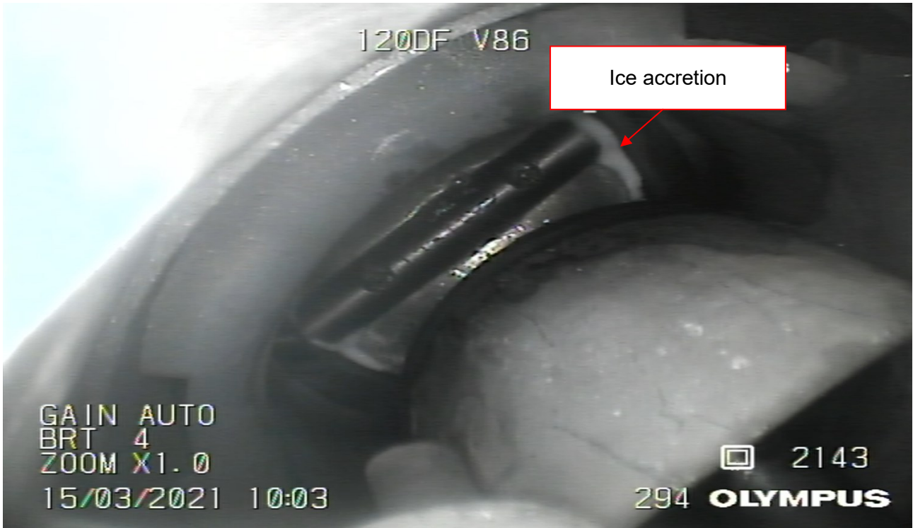
Figure 105: progress of icing => time designated t_{0+4min} Source: BEA
