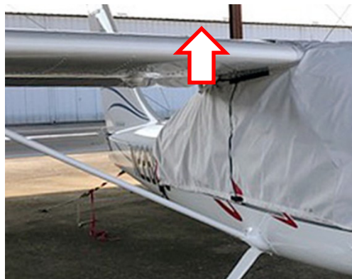
Figure 215: position of the temperature and relative humidity measurement sensor Source: BEA
