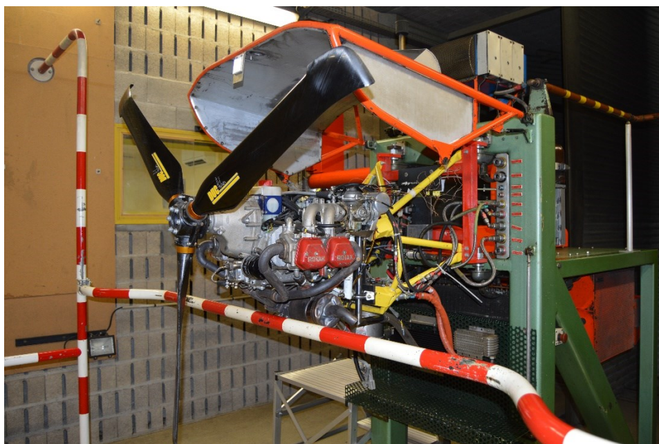
Figure 224: Rotax 914 engine at the test stand
