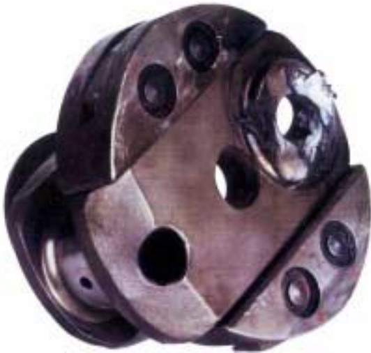
Face of rupture near M5/M6 arm
