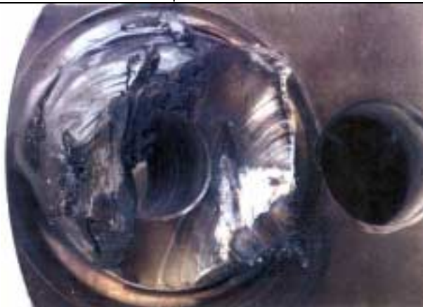
Rupture on rod journal No. 5 arm M5/M6 connection
