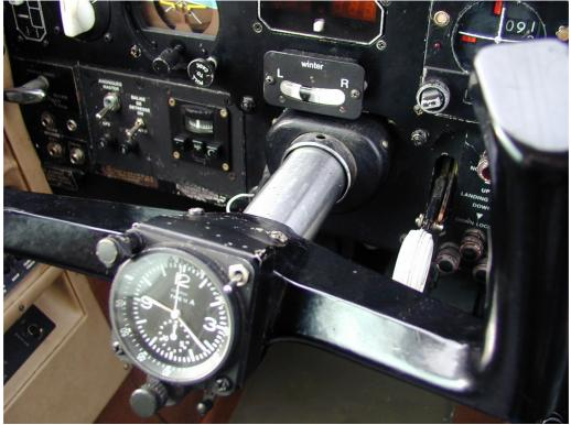
The wheel is thus maintained in a horizontal position, the ailerons remain in a more or less neutral position and the elevator is deflected down. No use of instruments or vital controls is affected by the presence of the locking device. The wheels on the accident aircraft were equipped with clips designed to hold the takeoff or landing charts. The presence of such a card tends to hide the metal plate. According to the crew's statements, no charts were in this position during
