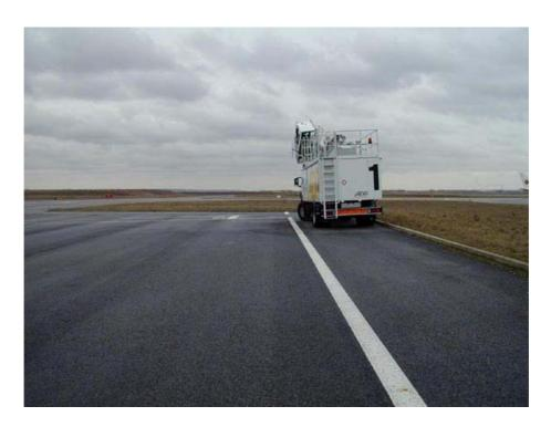
When vehicles are positioned beyond the markings, their position allows a Boeing 747-400 to pass with a lateral margin estimated at about ten meters, as shown in the photo.
