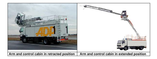
When the arm is retracted, the cabin can be in a high position (during use) or in a low position (during vehicle movements). The overall height of the vehicle is then 5.20 m and 4.10 m respectively. At the time of the collision, the cabin was in the high position, with the arm retracted.
