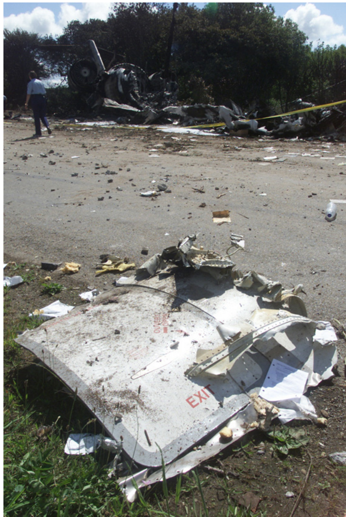
Forward right service door
