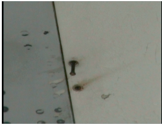
Example of a loose screw on a lower wing panel
