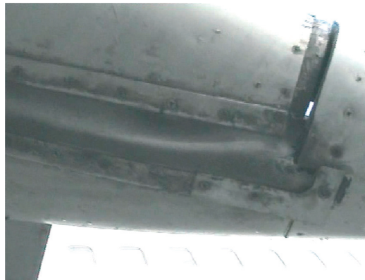
Example of the fairing of a flap guide rail that had come loose because certain rivets were missing
