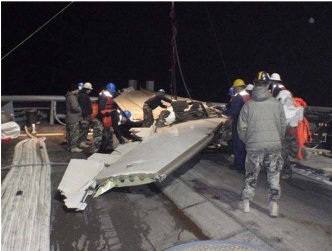
Figure 9: Recovery of the Stabilizer Section
