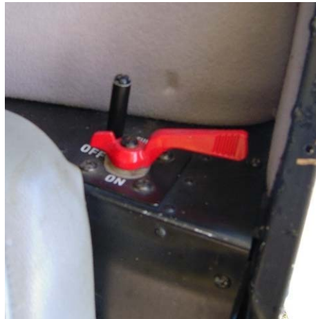
Position of the fuel cock observed in the wreckage
