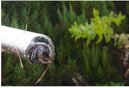
Drive shaft on the TGB side
