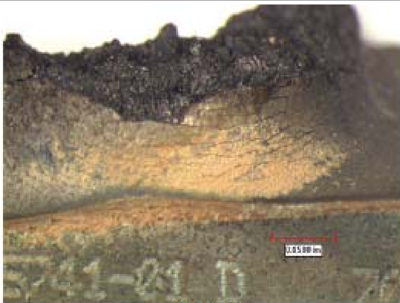
Photo No. 48 Multiple cracks parallel to the fracture surfaces
