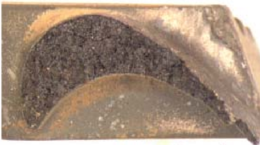
Photo No. 47 Typical condition of the CT blade fracture surfaces:
