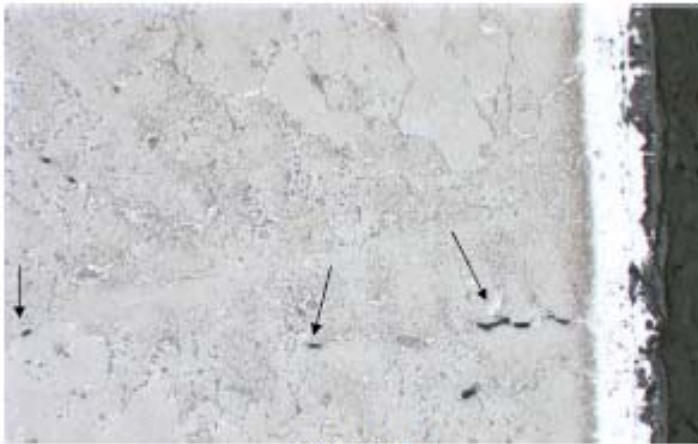
Photo No. 51 Blade No. 47 showing microvoids
