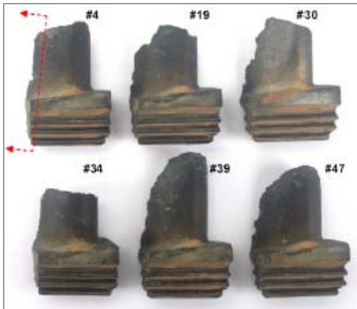
Photo n° 49 Six blades chosen for metallographic examination
