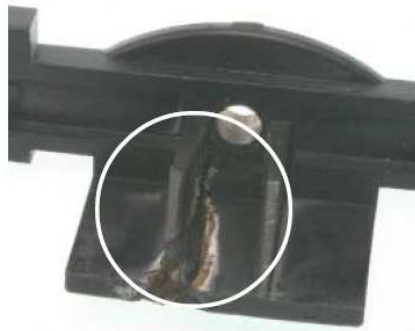
Unacceptable (Developing bearing bar failure)
