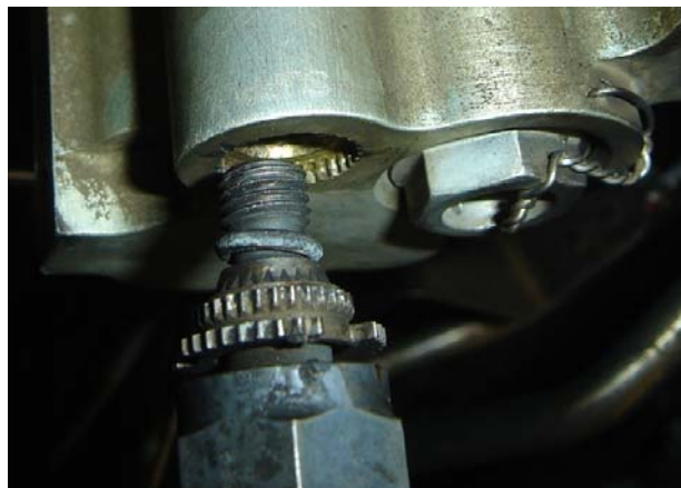
Disconnected OBV connector external damage
