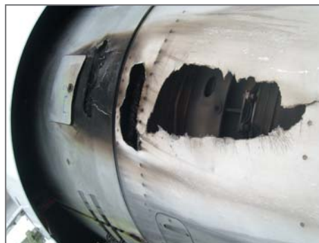
External damage to engine
