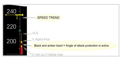
The low energy "SPEED SPEED" warning is an aural warning that indicates to the pilot that the total energy of the aeroplane is lower than a threshold below which the thrust must be increased to maintain a climbing flight path. This warning is available in configurations 2, 3 and FULL. It is inhibited above a height of 2,000 ft. During the incident, the triggering conditions for this warning were not met.
