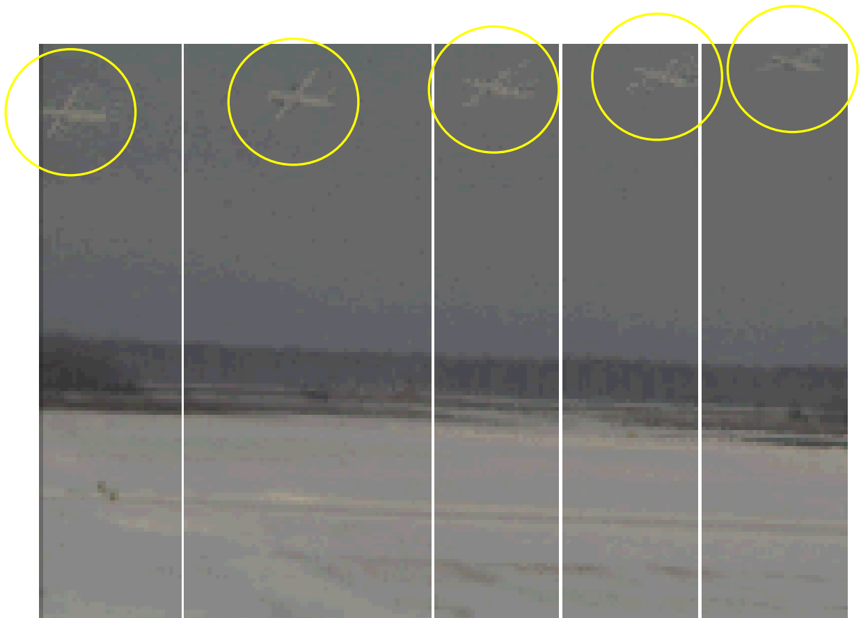
Figure 28. The trajectory of the A/C after the takeoff with developing left bank and descent
