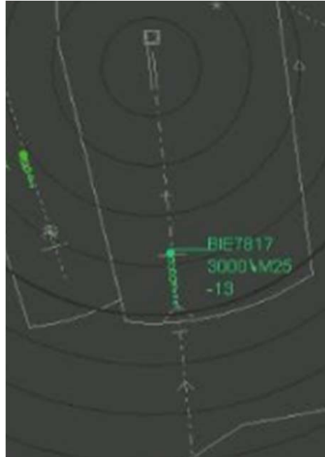
BIE7817 – crossing FAF (6.9 NM) – Radar: ground speed of 250 kts (CAS[FDR] = 206 kt, GS[FDR] = 241 kt)
