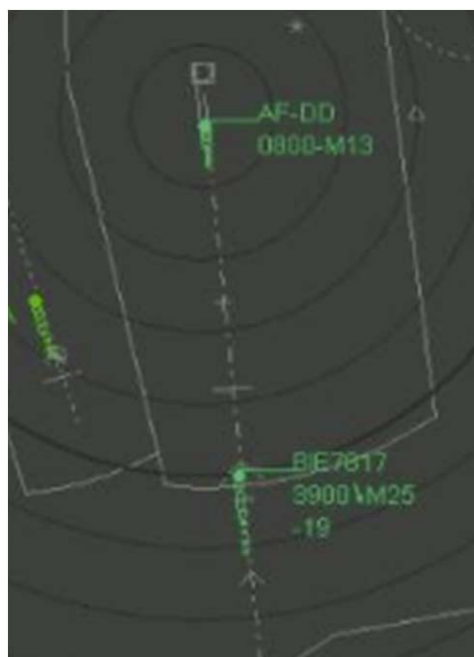
BIE7817- crossing 10 NM Radar: ground speed of 250 kts (CAS[FDR] = 222 kts, GS[FDR] = 251 kts )
