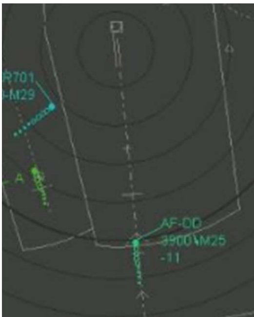
AF-DD - crossing 10 NM Radar: ground speed of 250 kts (CAS[FDR] = 220 kts, GS[FDR] = 249 kts)
