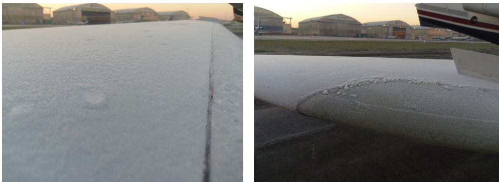
Figure 9 - Roughness on a wing contaminated by frost
