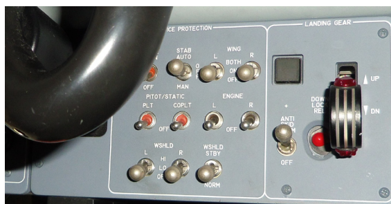
Figure 3 – ICE PROTECTION panel
