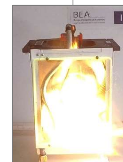
Oxygen box assembly catches fire
