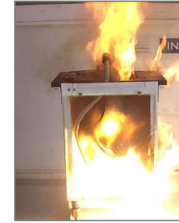
Fire escapes from oxygen box
