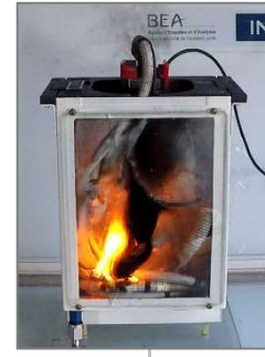
Fire spreads to harness and Nomex protection of hose
