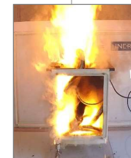
Fire escapes from oxygen box
