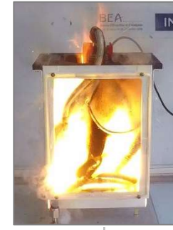
Oxygen box assembly catches fire
