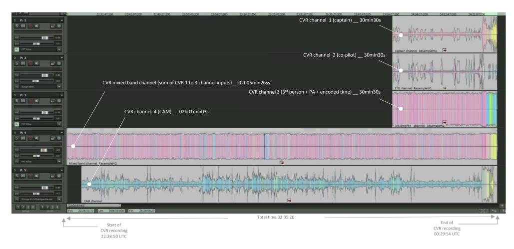
Note: the CVR data was synchronised (using the UTC time of the FDR) based on the information triggering the various warnings and the radio communication times recorded by the control services (ATC).
