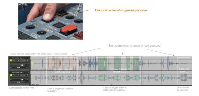
Pressing the pushbutton twice in quick succession generated in all the cases, a minimum interruption of **0.9 s** in the leaking noise to within the accuracy of the measurement.
