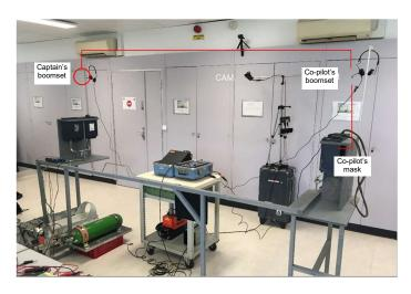
The complete A320 cockpit oxygen system assembly was taken from an aeroplane and set up in the laboratory.
