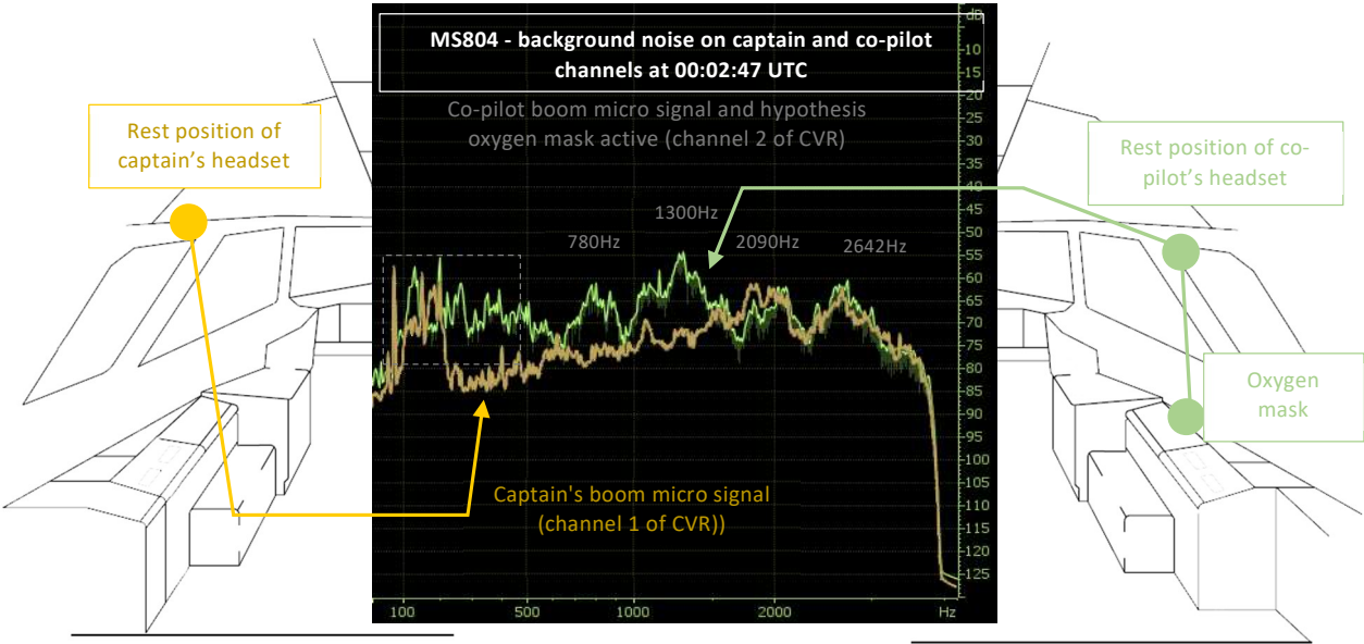
Figure 19: comparison of noise spectrum picked up by captain’s and co-pilot’s boom mikes
