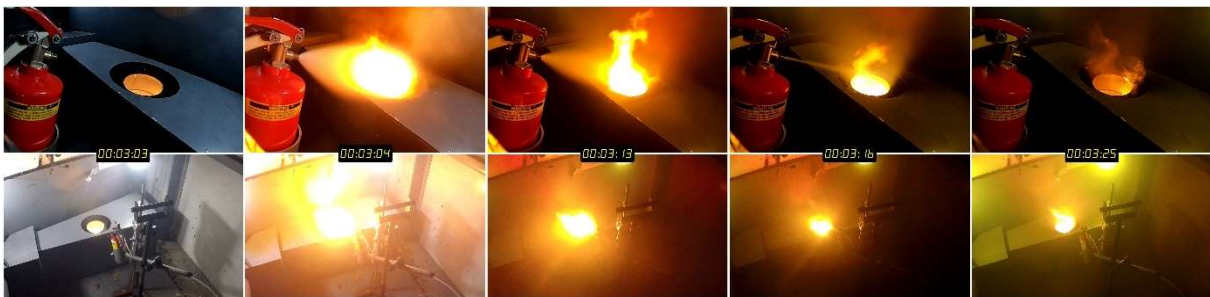
Figure 50: extinguisher_02 test - video sequence (source: BEA)
