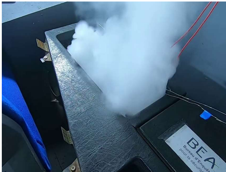
Figure 27: release of smoke during Lithium_Battery_05 test
