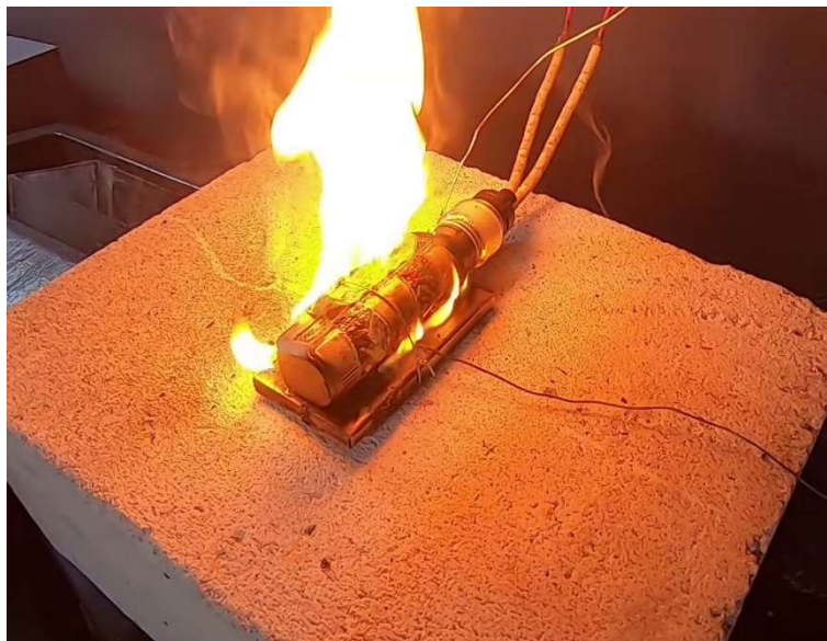
Figure 26: visible flames during Lithium_Battery_07 test
