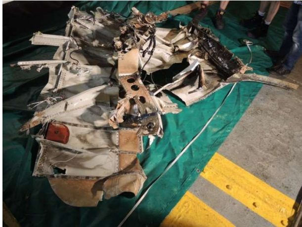
Figure 16: cockpit debris showing black deposits (source: BEA/EAAID)
