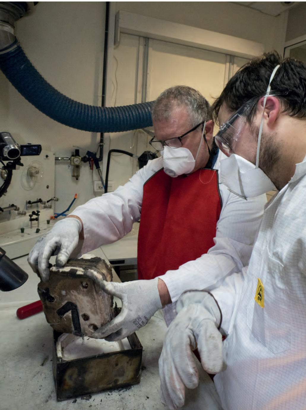
When analysing a flight recorder damaged in an accident, it may be necessary to analyse each electronic circuit, and repair them if necessary, before downloading and analysing the data.
