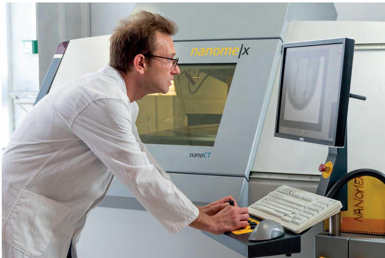
X-ray tomograph analysis of a part
