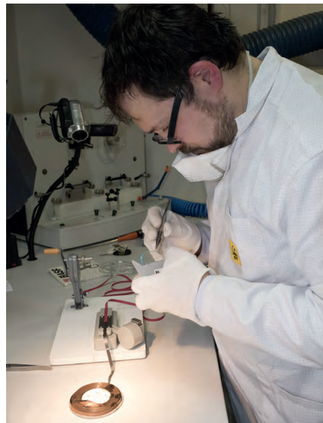
When analysing a flight recorder damaged in an accident, it may be necessary to analyse each electronic circuit, and repair them if necessary, before downloading and analysing the data.
