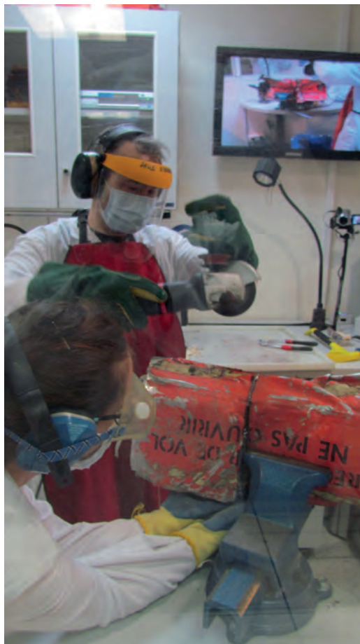
Opening a recorder under the eye of the camera in order to certify the operations.
