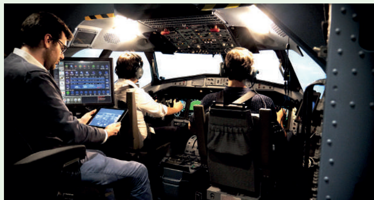
Flight simulation training device: the human factor is analysed in order to be incorporated in the safety investigations.
