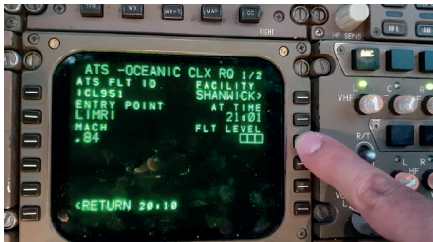
ACARS (Aircraft Communications, Addressing and Reporting System) is a digital communications system used on aircraft to send and receive messages in text format between aircraft and ground stations.
