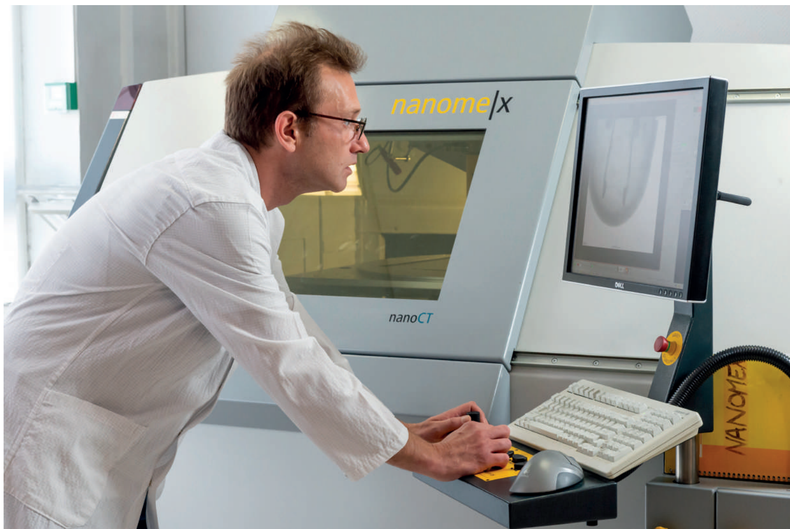
X-ray tomograph analysis of a part
