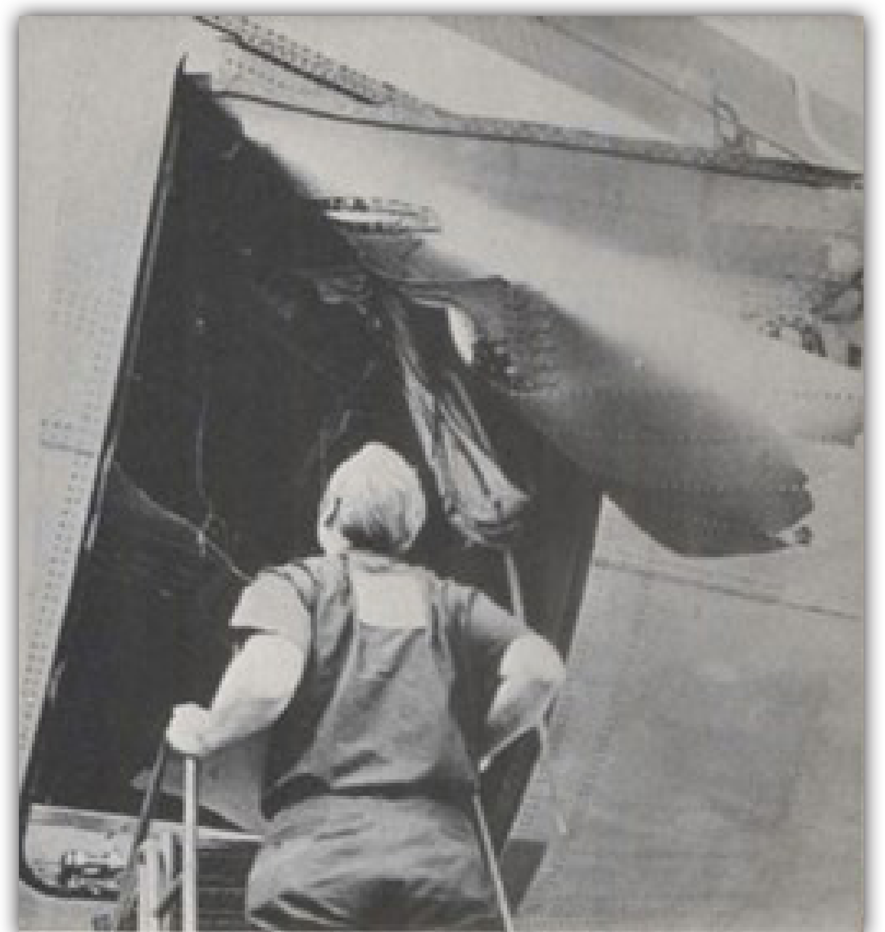
Photo of the American Airlines DC-10 door from the accident in 1972.
