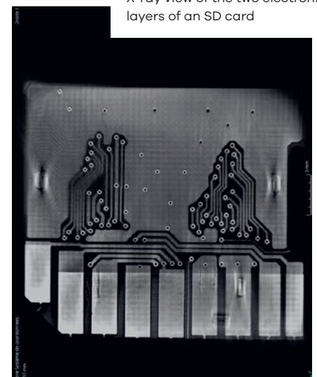
X-ray view of the two electronic layers of an SD card
