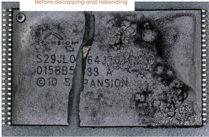
Before decapping and rebonding
