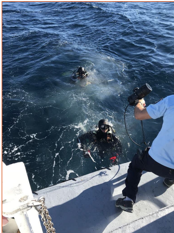
BEA taking part, on 09 September 2022, in a test carried out in Antibes by the CNING (Centre National d’Instruction Nautique de la Gendarmerie) and the Gendarmerie on a device designed to locate transmitters attached to flight recorders.
