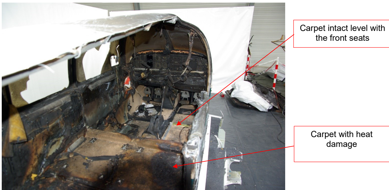
Figure 17: Cockpit after cutting the fuselage and removing the seats Source: BEA
