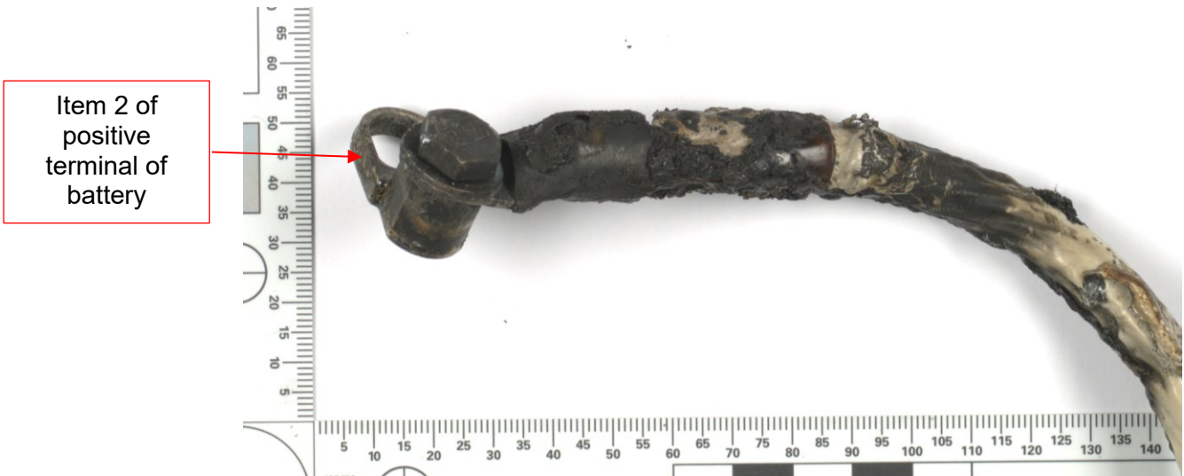
Figure 66: Conductor associated with positive terminal of battery with connector Source: BEA
