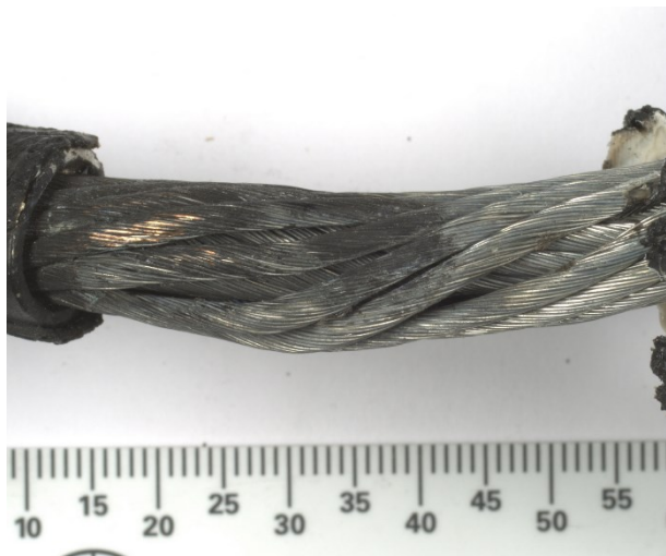
Figure 68: Deformation of strands making up conductor Source: BEA
