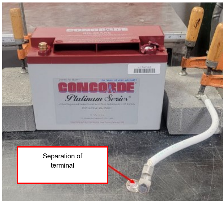
Figure 74: Separation of parts 1 and 2 of terminal Source: Concorde Aircraft Batteries
