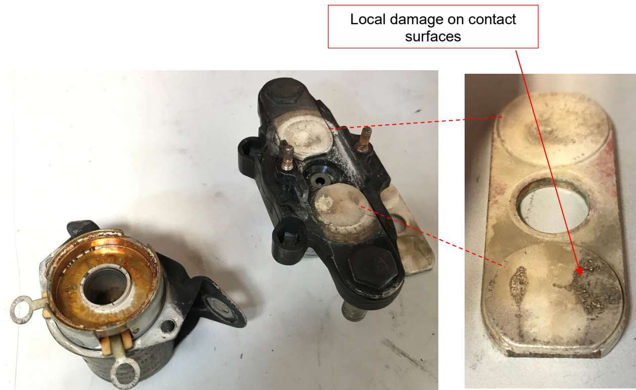
Figure 136: Master solenoid disassembled in the BEA laboratory
