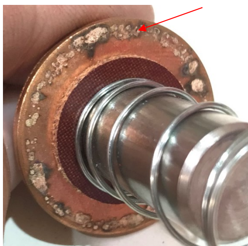
Figure 159: Signs of electrical arcs in operation Source: BEA
