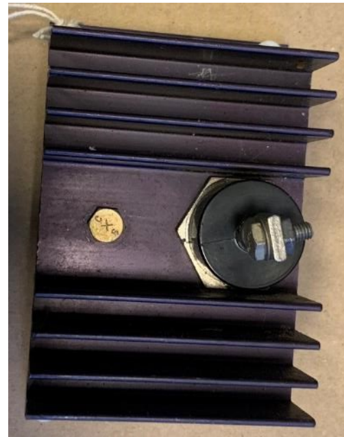
Figure 95: Diode device supplied by Concorde Aircraft Batteries to the BEA 19 Source: BEA
