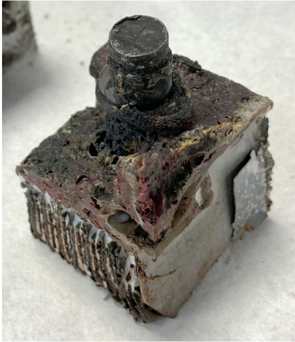
Figure 57: Positive terminal of battery Source: BEA
