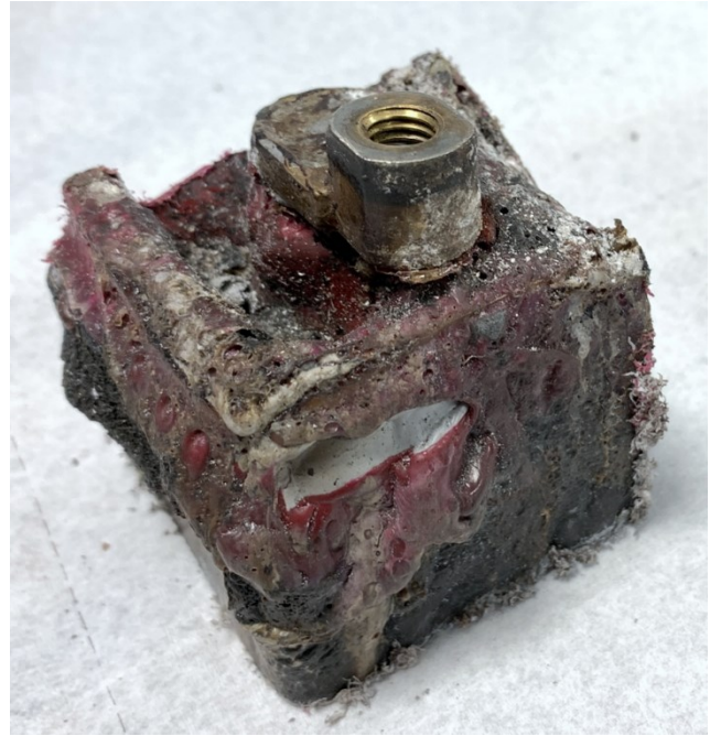
Figure 58: Negative terminal of battery Source: BEA
