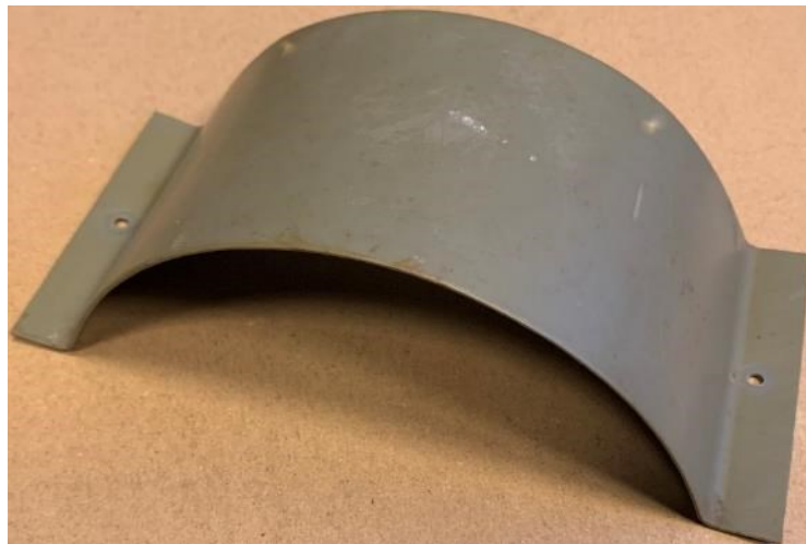
Figure 96: ABS cover supplied by Concorde Aircraft Batteries to the BEA Source: BEA
