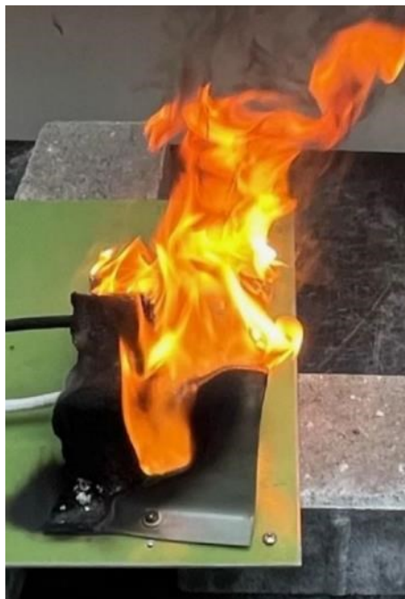
Figure 125: Burning ABS cover Source: Concorde Aircraft Batteries
