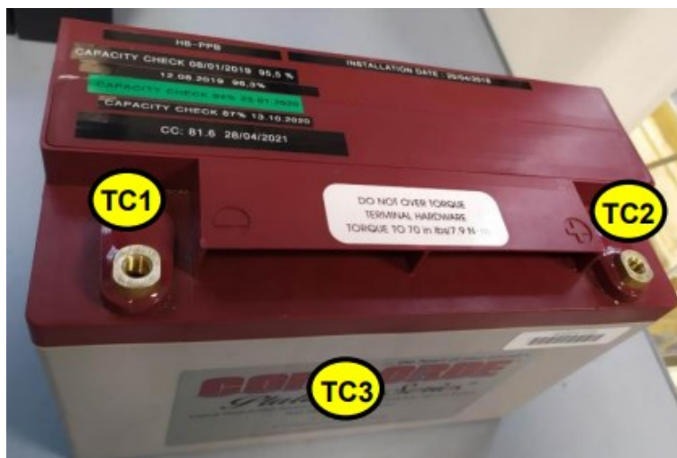
Figure 81: Position of thermocouples on battery Source: INES CEA
