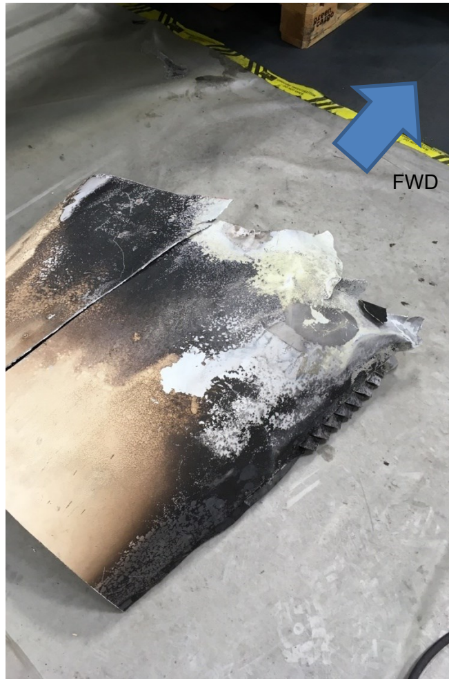
Figure 11: Area where the external paint on the sheet was damaged or destroyed (upper part of the aeroplane) Source: BEA
