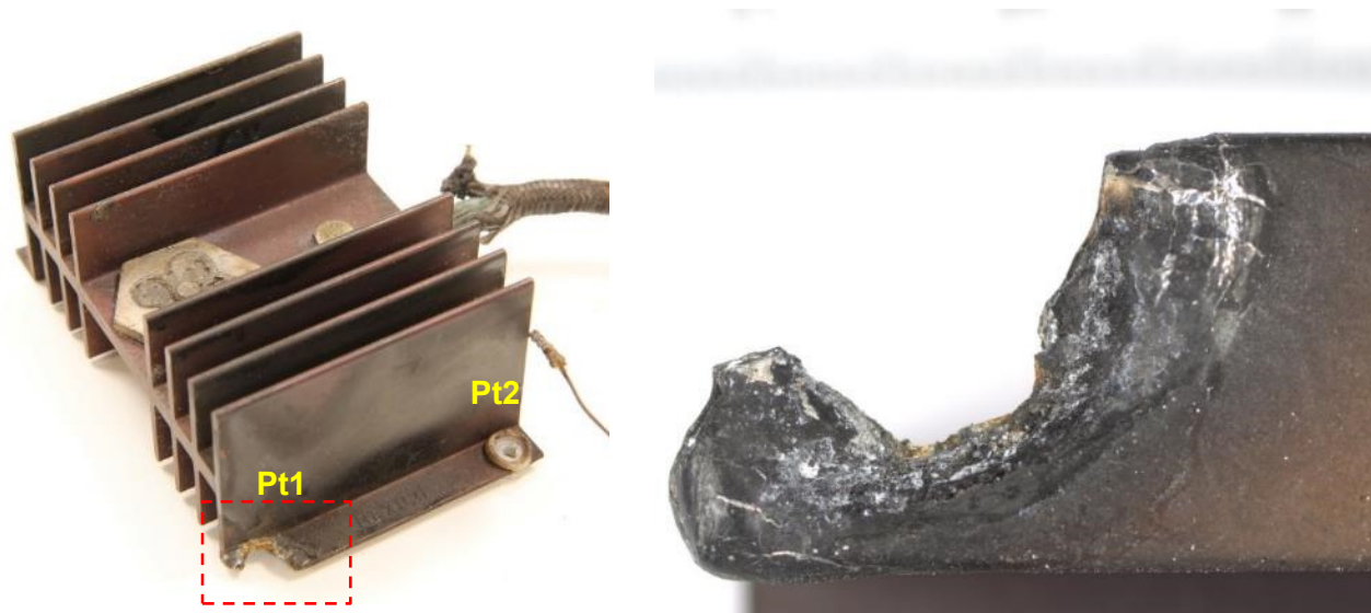
Figure 107: metal cooler and detail view of damaged area
