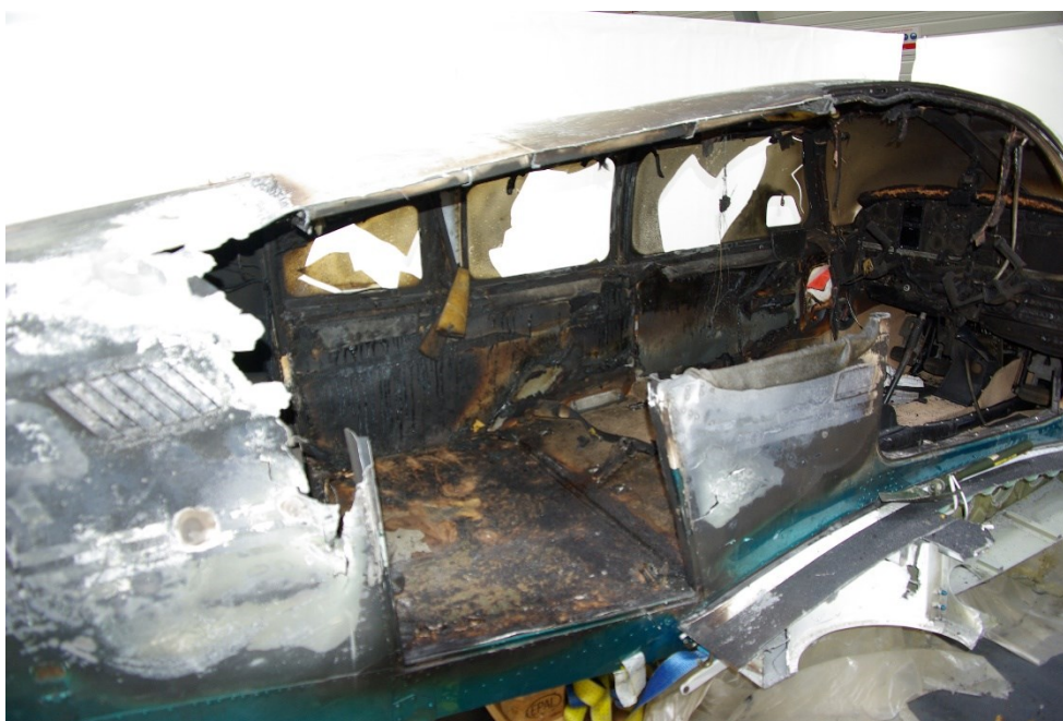
Figure 18: Cockpit after cutting the fuselage and removing the seats Source: BEA
