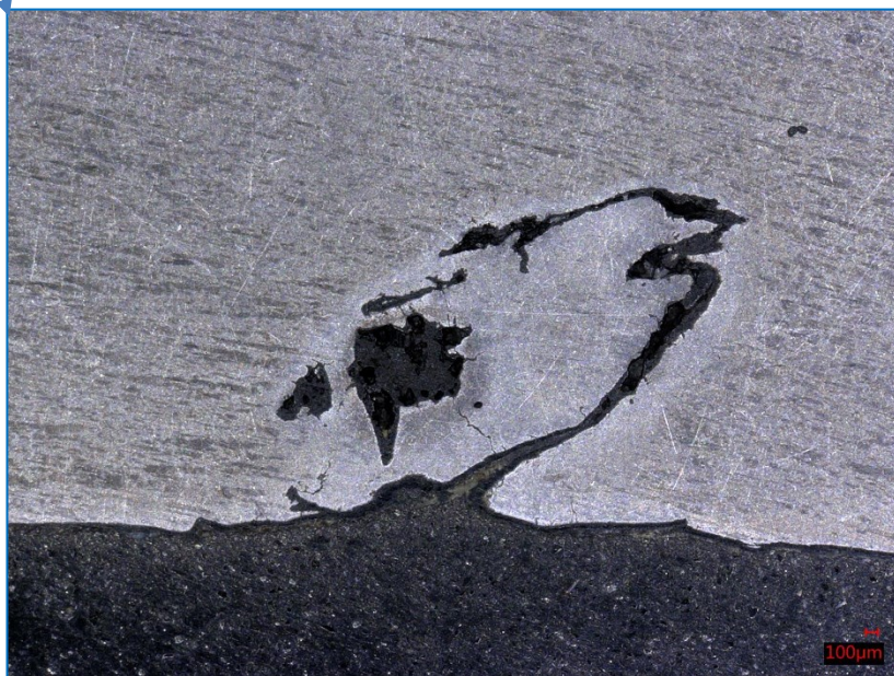
Figure 64: Arc type damage within positive terminal Source: BEA
