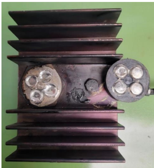
Figure 127: Separation of diode bridge from metal cooler Source: Concorde Aircraft Batteries
