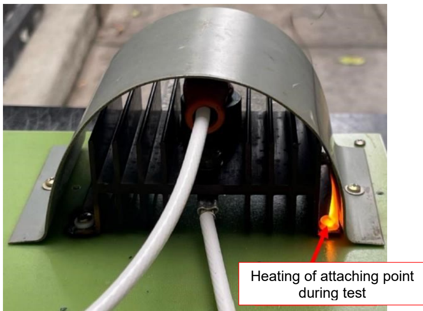
Figure 124: ABS cover in position with attaching point subject to intense heat Source: Concorde Aircraft Batteries
