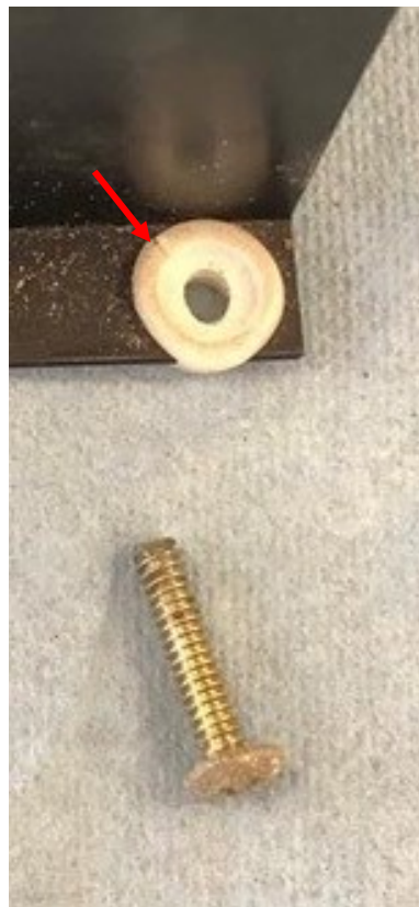
Figure 112: Cracked upper flange of insulating washer Source: maintenance workshop for HB-PPB
