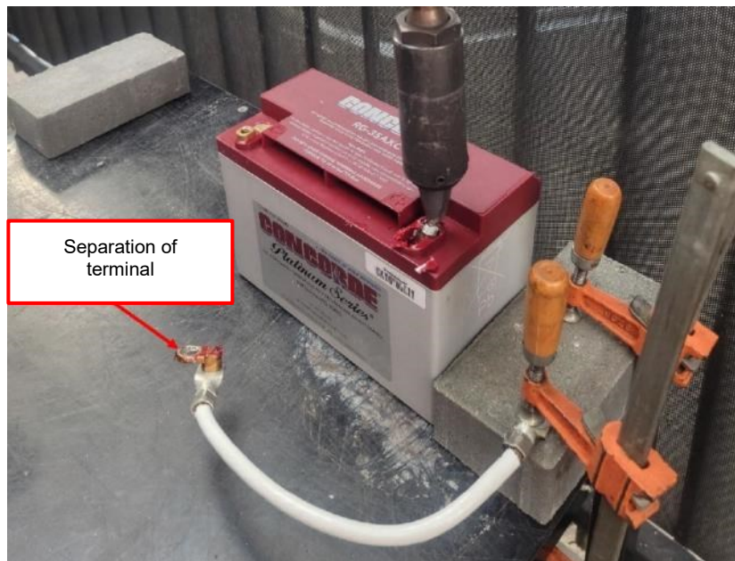
Figure 71: Separation of parts 1 and 2 of terminal Source: Concorde Aircraft Batteries
