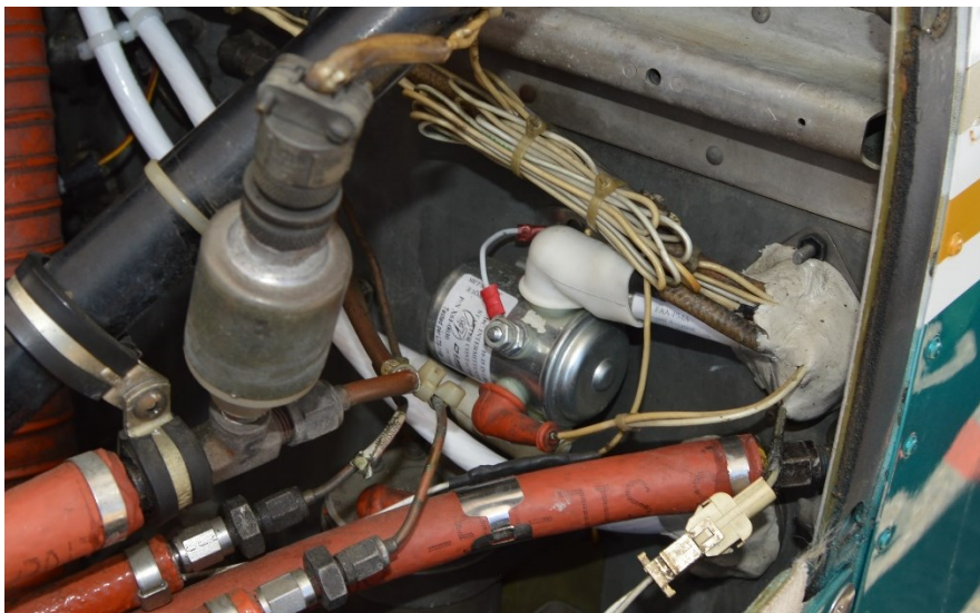
Figure 153: Starter solenoid in position in the engine compartment on the firewall Source: BEA
