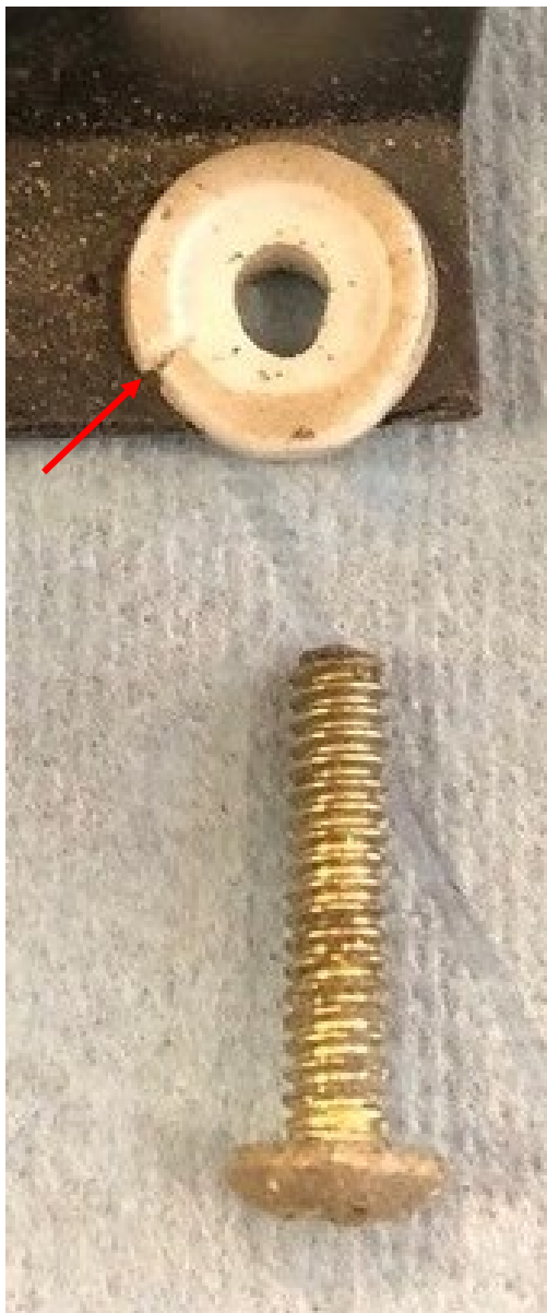
Figure 111: Cracked upper flange of insulating washer Source: maintenance workshop for HB-PPB
