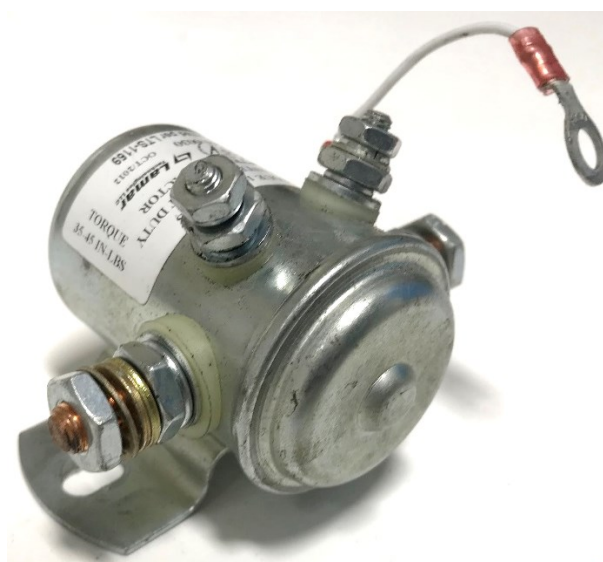
Figure 155: Starter solenoid removed from aircraft Source: BEA
