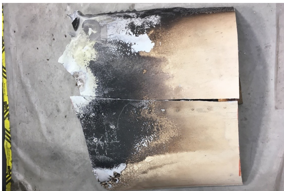
Figure 10: Area where the external paint on the sheet was damaged or destroyed (upper part of the aeroplane) Source: BEA
