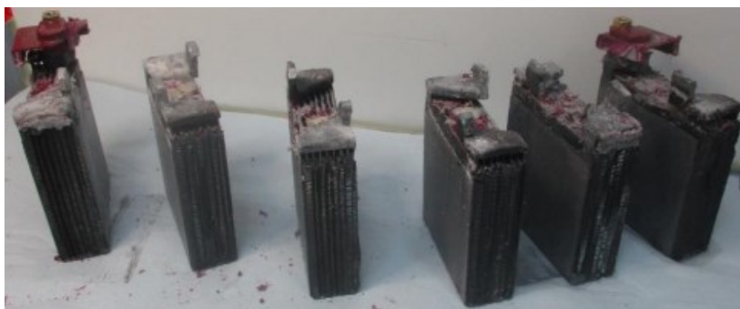
Figure 89: Cells making up battery Source: INES CEA
