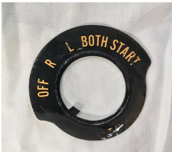
Figure 149: Start-up switch plate indicating the five possible positions Source: BEA
