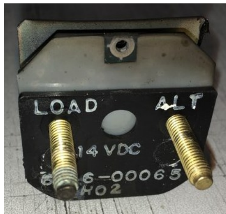
Rear side of ammeter
