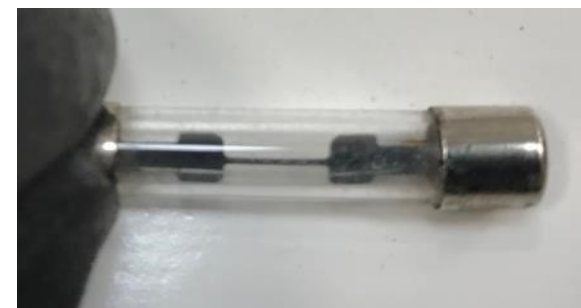
Figure 106: 5A fuse associated with diode device Source: BEA
