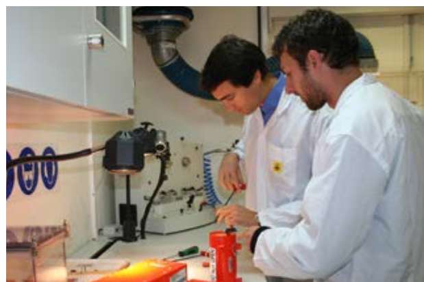
Read out and analysis of a flight data recorder at BEA
