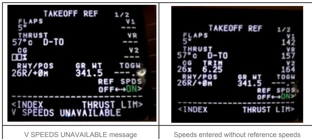
Figure 3: Screenshots of FMS Take-off parameters close to those of the incident
