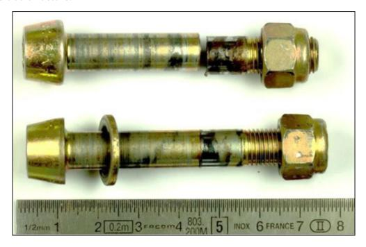
Figure 6: central attachment bolt, left bolt above, right bolt below
