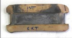
Figure 7: right main landing gear flange and leather spacer
