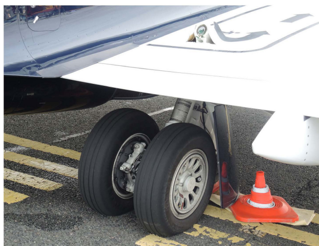
Figure 6: view of right main landing gear broken at top
