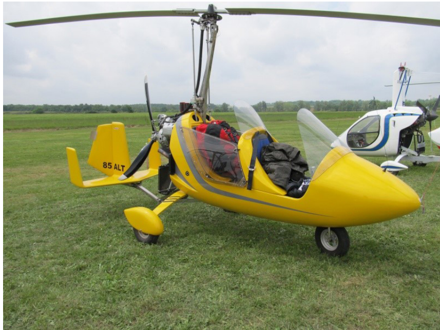
Figure 2: photo of the gyroplane before installing the cockpit canopy and modifying the tail assembly
