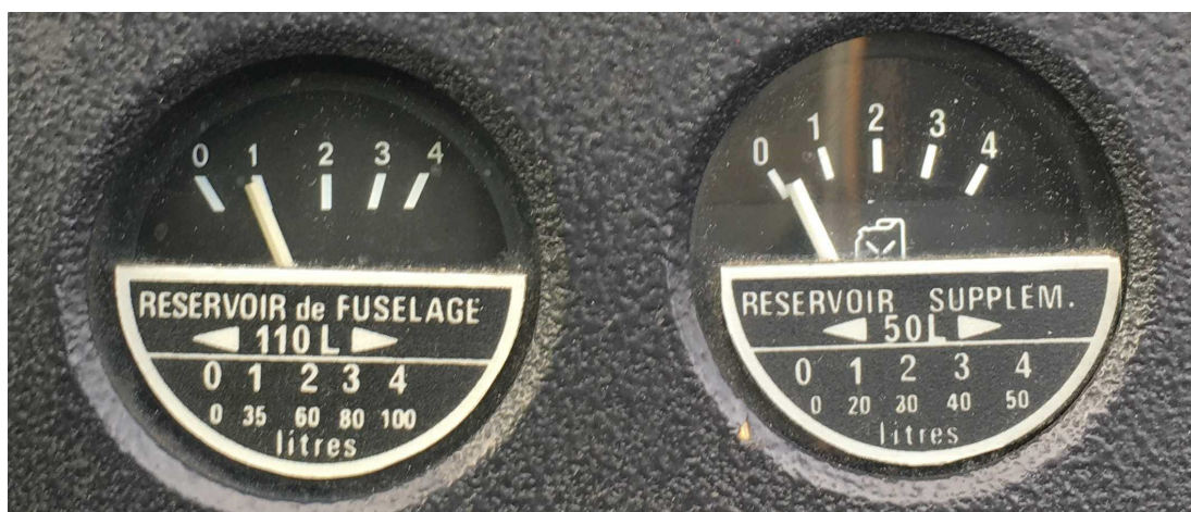
Figure 4: position of the needles on power-up with both tanks empty
