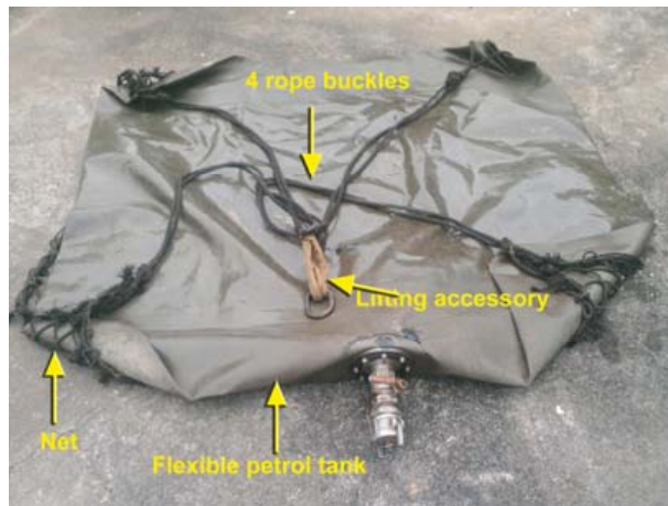
Figure 2 - assembled load and lifting accessory
