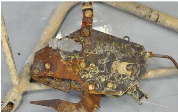
Figure 9 - burnt load releaser
