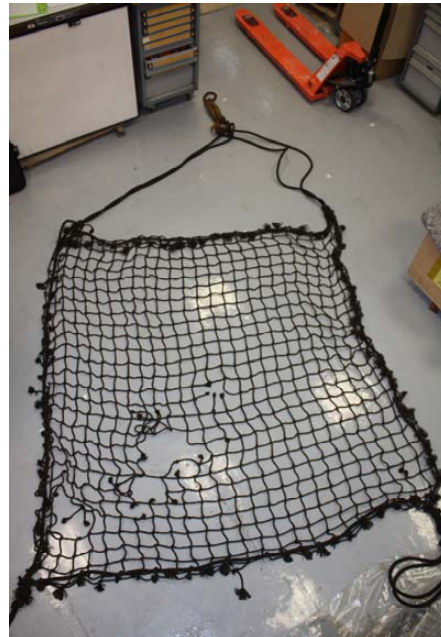
Figure 8 - damaged net attached to the lifting accessory via two buckles
