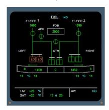
Figure 2: simulation of the FUEL page after the "FUEL L TK PUMP 2 LO PR" warning
