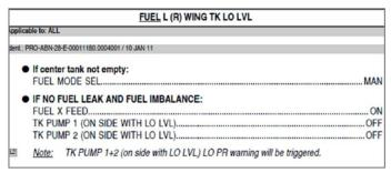
Figure 4: "FUEL L(R) WING TK LO LVL" SOP(9)
