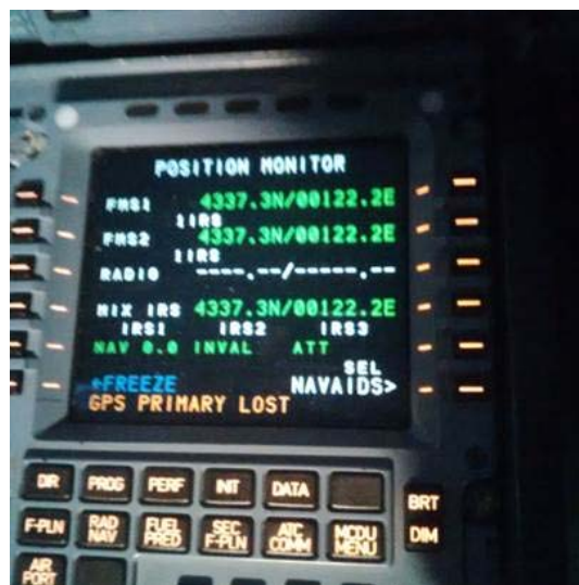
Figure 4: Example of POSITION MONITOR page. Photo taken in simulator. Note the IRS modes
