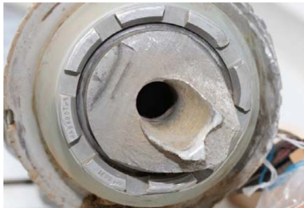
Figure 2: fracture pattern on blade No.2 pre-load bolt
