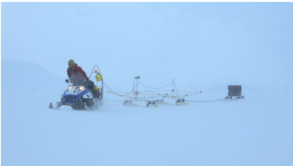
Fig. 35: Snowmobile towing SnowTEM during the test in Zermatt in low visibility conditions in a snow storm
