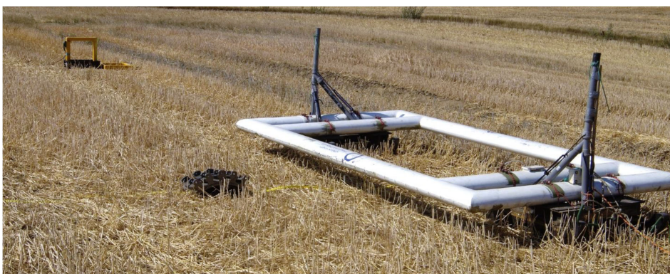
Fig. 29: Picture of test setup: test hub placed 2 m from center of transmitter frame
