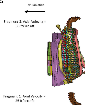
Fig. 4: Simulation results of the fan hub bore to rim rupture scenario, consistent with damage observed on engine
