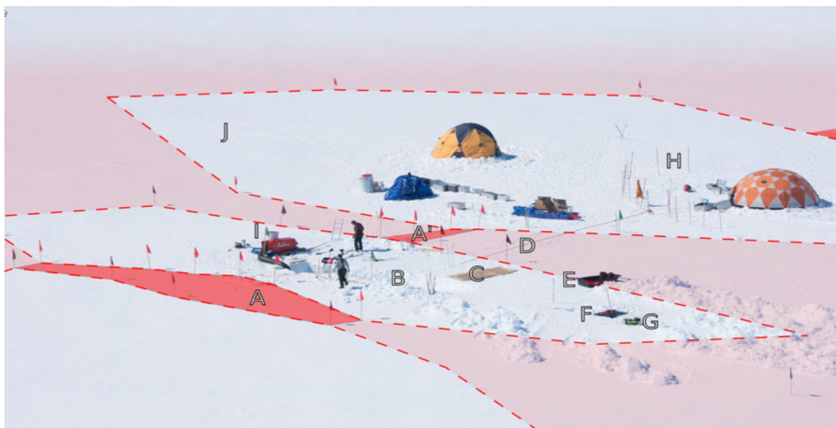
Fig. 42: Photograph from helicopter of excavation work-site as described in (Mankoff, et al., 2020). (A and A') Dark red graphic overlays between flags mark known crevasse locations as detected by GPR and DGNSS. Dashed lines enclose safe areas and pink marks unsafe areas defined with GPR data, the UHF basemap (Fig. 21), extensive snow probing and crevasse location uncertainty with distance from known crevasse locations. (B) Ramp out of pit. (C) Plywood used to cover pit overnight to prevent drifting snow filling. (D) Safety rope bridging crevasse between the northern (far) camp island and the southern (near) work island. (E) Sled. (F) Winch and winch platform. (G) Generator used to power winch. (H) Bamboo poles marking polar bear alarm trip-wire surrounding sleep tent. (I) Herman Nelson heater, hose and fuel barrel. (J) Helicopter landing zone. Photo by Austin Lines.
