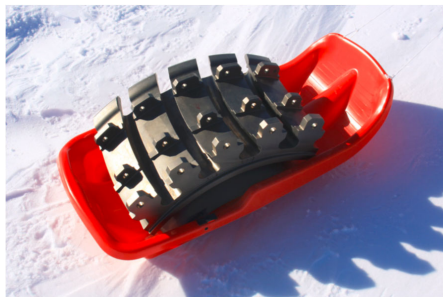
Fig. 48: part of a fan hub mock-up on its sledge, later referenced as “test hub” (left picture), and once buried (right picture)
