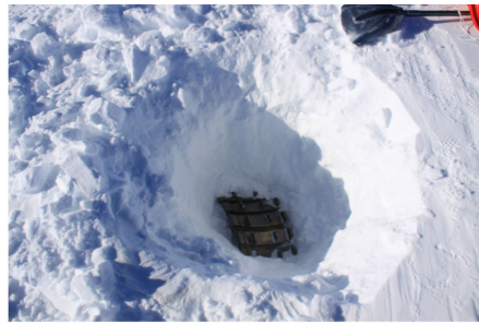
Fig. 48: part of a fan hub mock-up on its sledge, later referenced as “test hub” (left picture), and once buried (right picture)
