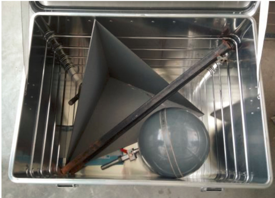
Fig. 46: trihedral and sphere in their transport crate
