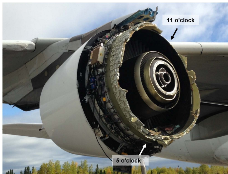
Fig. 17: side view of engine N° 4 on aircraft after landing
