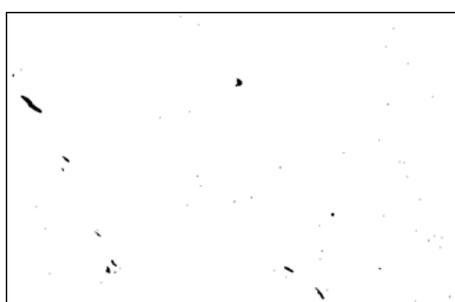
Figure 83: binary image, the result of the processing process. The inclusions are shown in black
