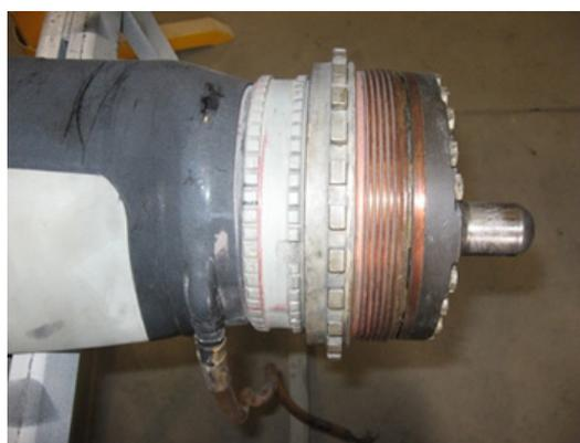
Figure 18: view of the complete blade bearing assembly
