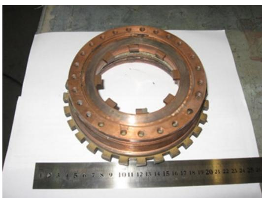
Figure 17: blade bearing
