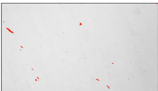
Figure 82: definition of the grey level threshold for identification of inclusions (in red)
