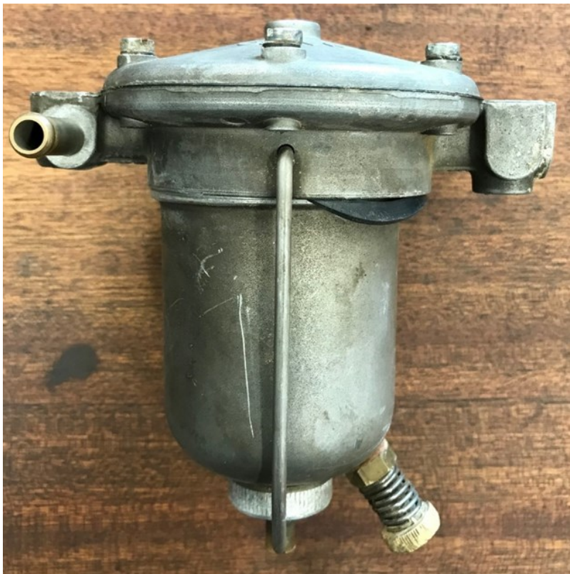
Figure 2: fuel filter, with pinched seal (source: BEA)
