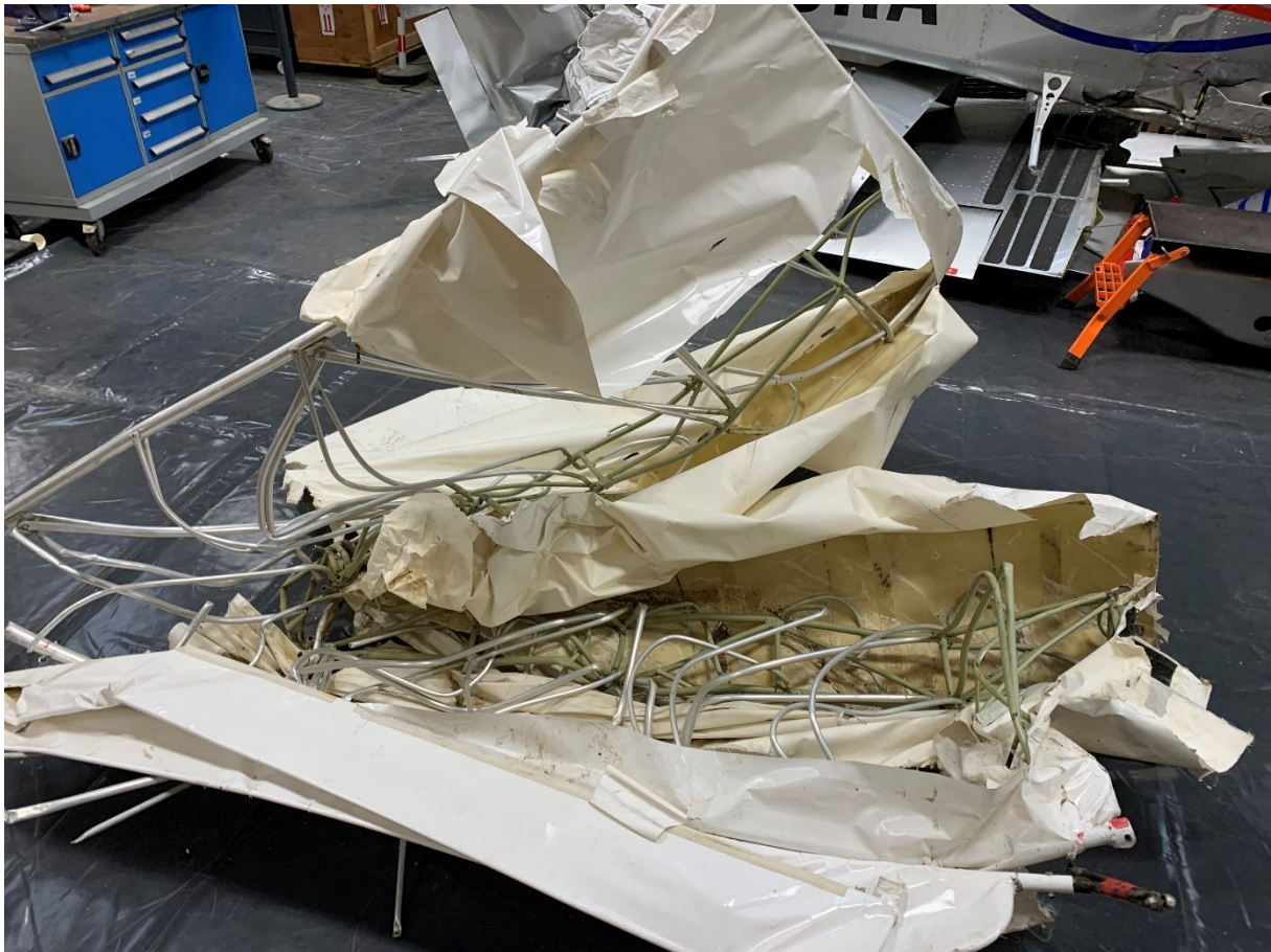
Figure 7: view of left wing of 03AEG with partial separation of aircraft fabric (source: BEA)
