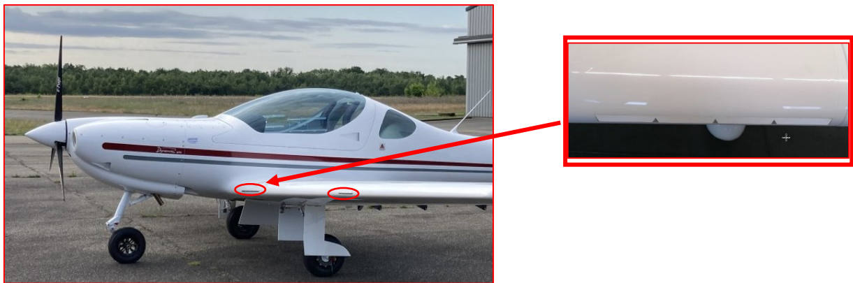
Figure 6: stall strips on a WT9 microlight (Source: Finesse Max)
