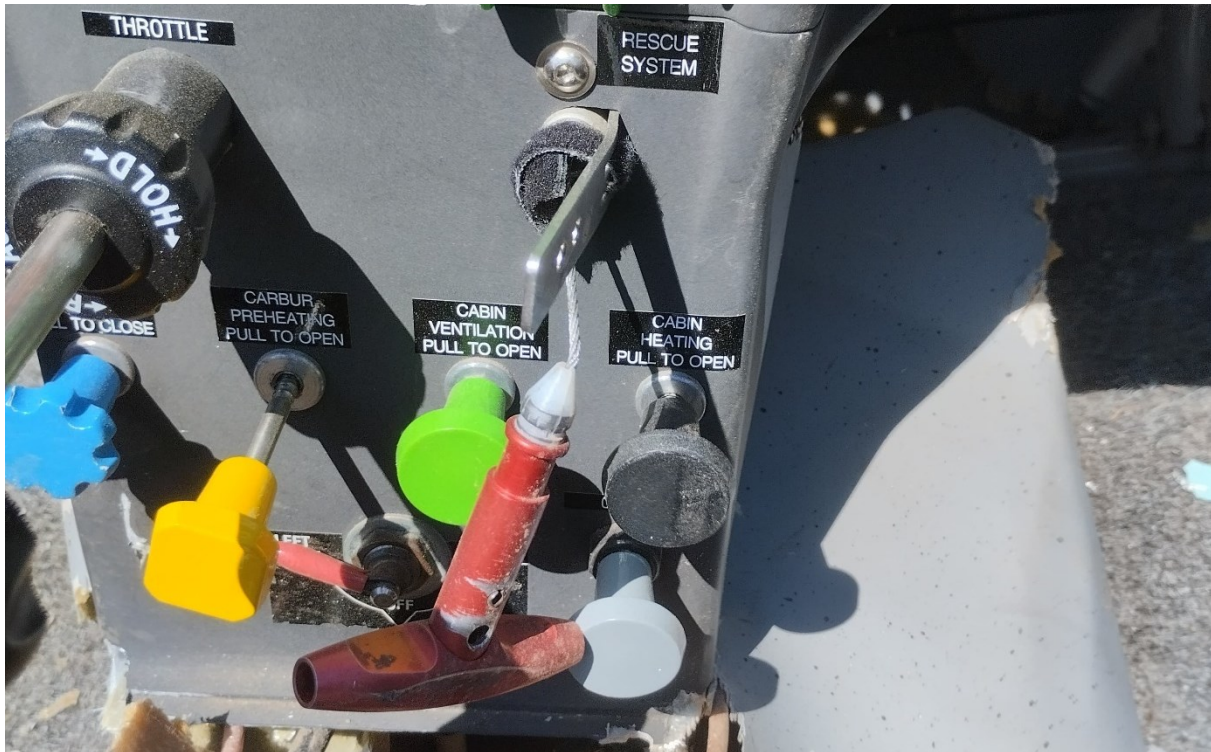
Figure 4: position of the airframe parachute handle after the accident (Source: BEA)
