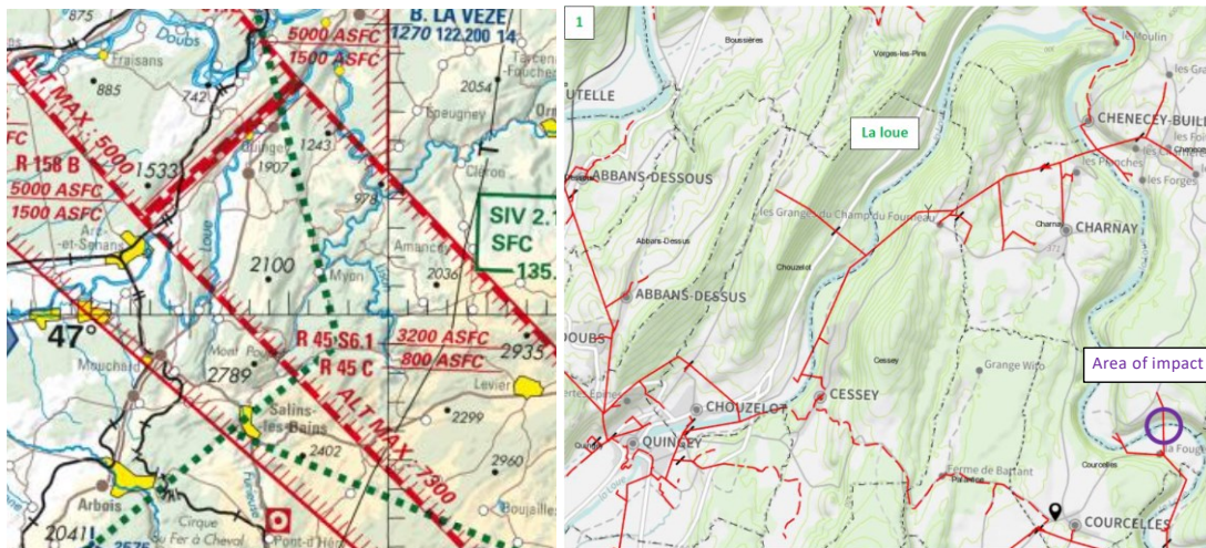
Figure 5: location of electrical power lines (sources: on left, IGN/ICAO map scale 1:500,000, on right Enedis)
