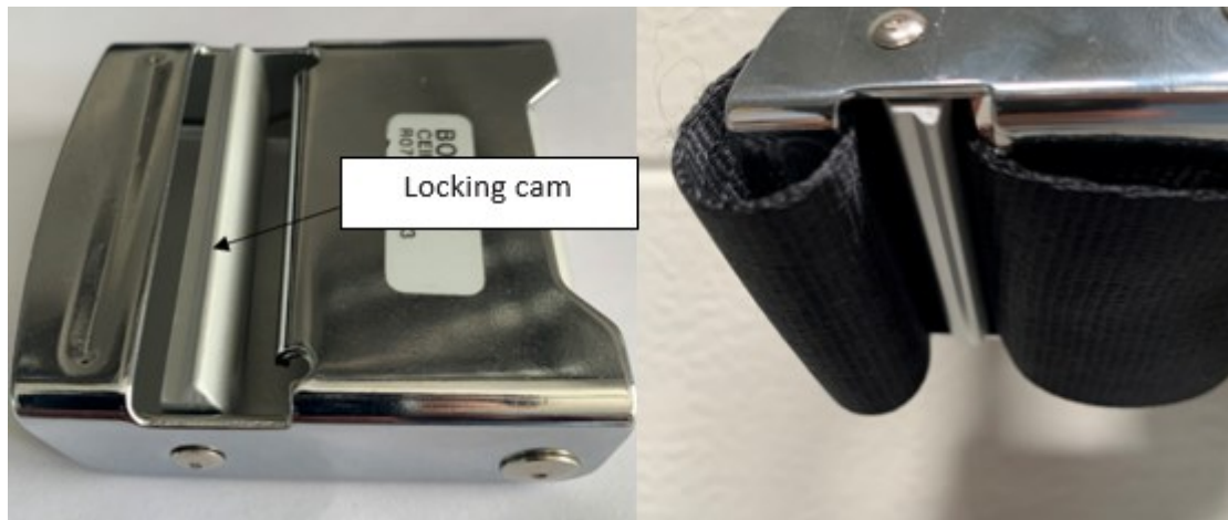
Figure 7: female metal buckle on the passenger's lap belt (source: BEA)
