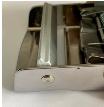
Figure 8: female metal buckle of pilot's lap belt (source: BEA)
