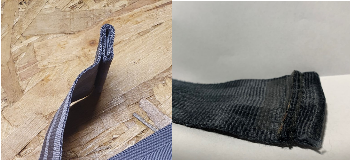
Figure 9: detail of webbing and hem: on LH side, Anjou Aéro strap, on RH side, strap assembled on Air Création microlight (source: Anjou Aéro/BEA)
