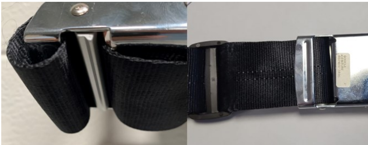
Figure 10: on LH side, correct assembly of strap on metal female buckle, on RH side, reverse assembly (source: BEA/ Air Création)
