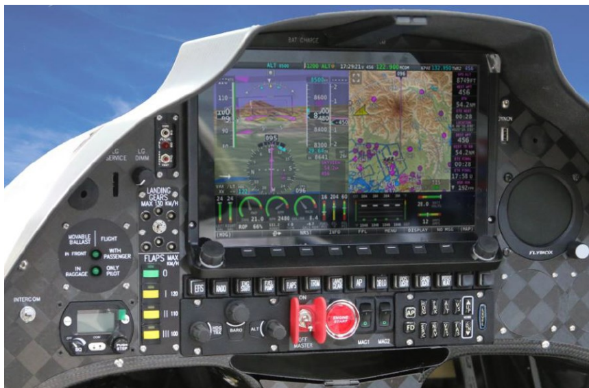
Figure 4: front instrument panel of a Shark 600F (source: Flight manual, Shark Aero)
