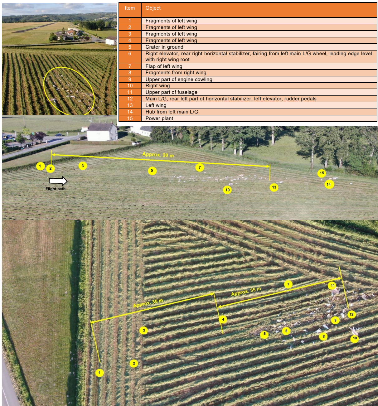
Figure 4: distribution of the microlight debris (Source: BGTA, annotated by the BEA)
