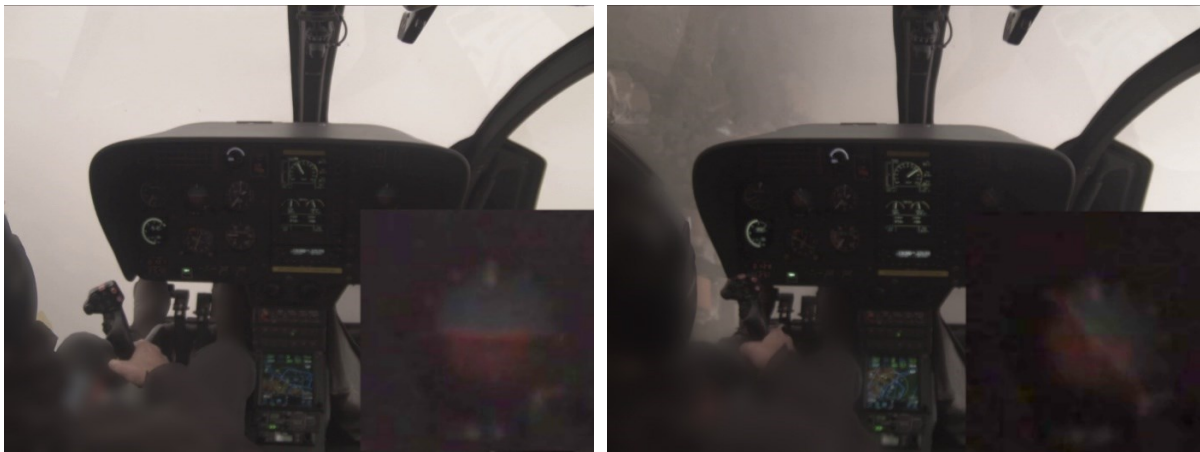
The LH image shows the absence of visual references, the helicopter is horizontal in level flight. The RH image corresponding to point 4 of Figure 8, shows that the external references are briefly visible (ground and houses on bottom left of image). At this point, the helicopter is in a left bank of around 50°.
